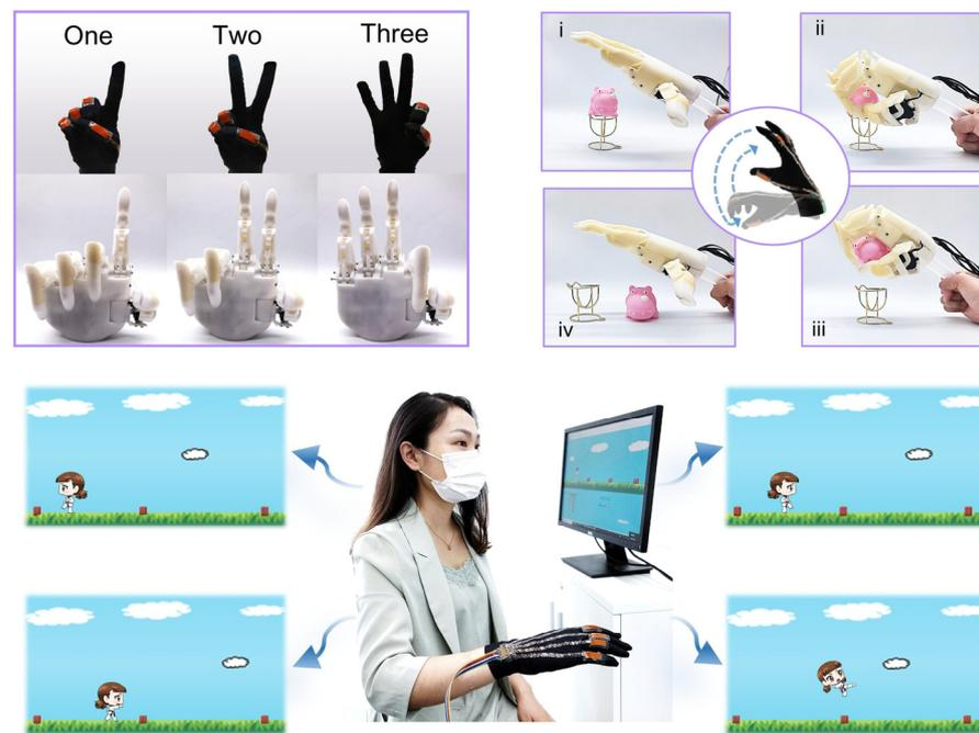
**Figure 6.** Human–machine interface applications of flexible and stretchable pressure sensors. Note that (i–iv) step process for grab object. (Reproduced with permission from Elsevier [107]).
