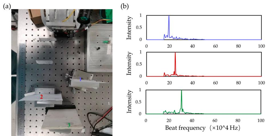
Figure 7. (a) Image of three targets placed at different angles and distances relative to the chip (b); FFT spectra computed from measured signal reflected from three targets scanned by OPA.
