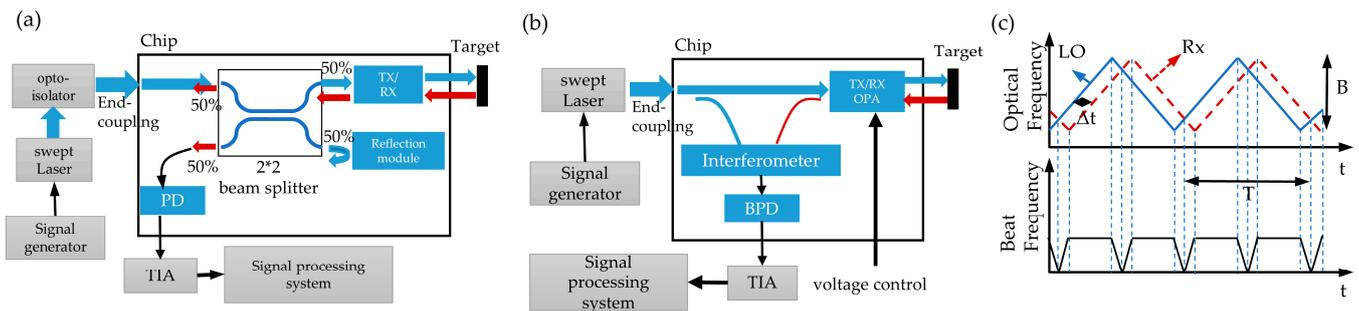
**Figure 1.** (a) Schematic diagram of on-chip coaxial FMCW LiDAR system built by  $2 \times 2$  beam splitter; (b) schematic diagram of on-chip FMCW LiDAR system with solid-state beam steering by interleaved coaxial optical phased array; (c) ranging principle.
