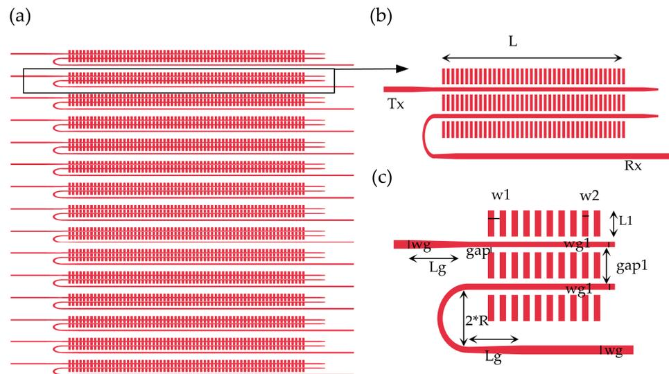
**Figure 3.** (a) Schematic diagram of interleaved coaxial optical phased array; (b) schematic diagram of interleaved coaxial antenna; (c) zoomed-in image of part of the antenna.
