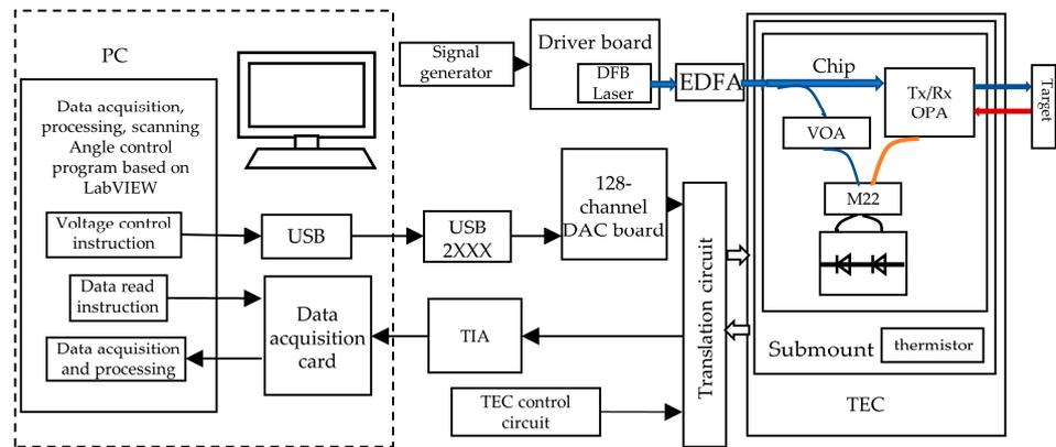
Figure 6. Test system for on-chip solid-state FMCW LiDAR.
