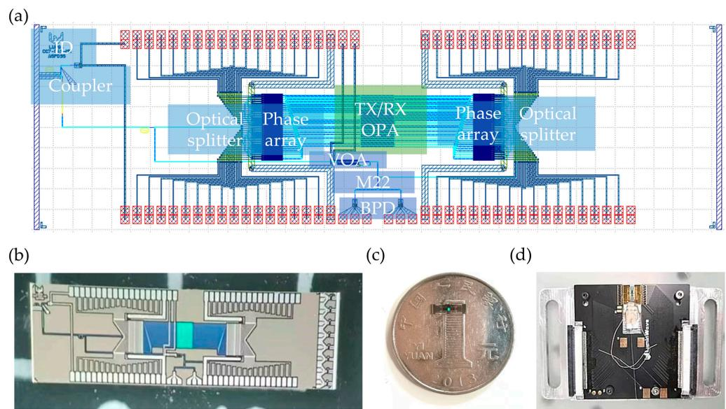
**Figure 2.** (a) Schematic diagram of the chip; (b) optical micrograph of the chip; (c) chip is placed on a one-yuan coin; (d) packaged system.
