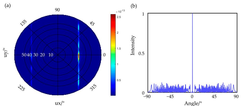
**Figure 4.** (a) Far-field distribution of a single antenna; (b) far-field distribution of an OPA with nonuniform array design.
