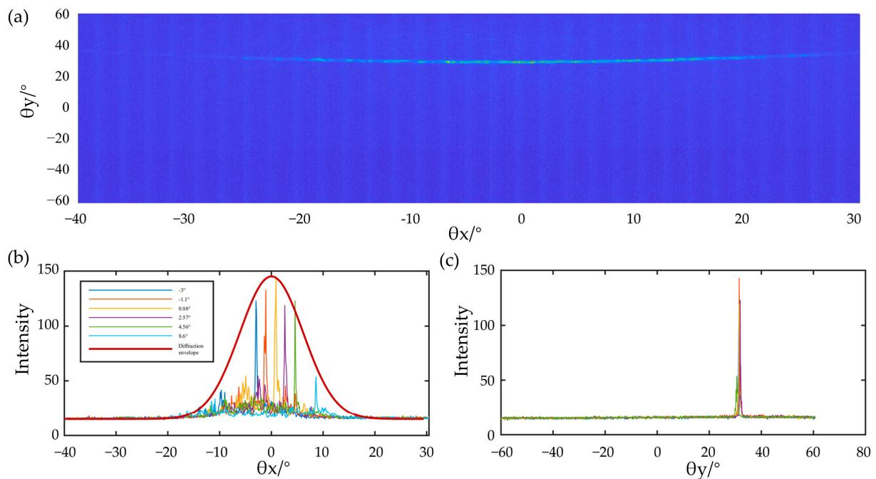
**Figure 5.** (a) Far-field distribution of the optical phased array when the emission optical phased array is not voltage applied to the phase shifter; (b) beam steering results by adjusting the phase shifters. Several scanned far-field intensity distributions in  $\theta_x$  direction represented by different colors; (c) corresponding far-field distribution in  $\theta_y$  direction.
