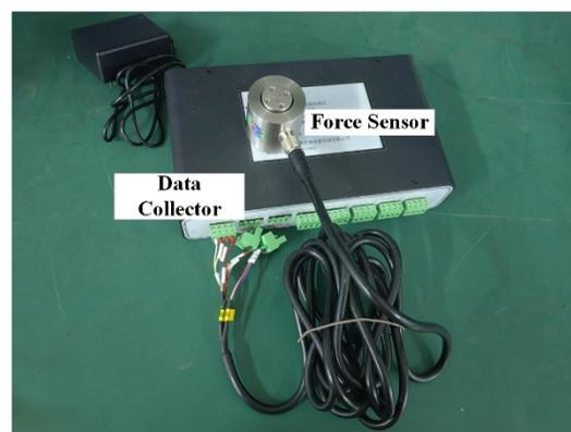
Figure 16. The 3D force sensor data measurement system.
