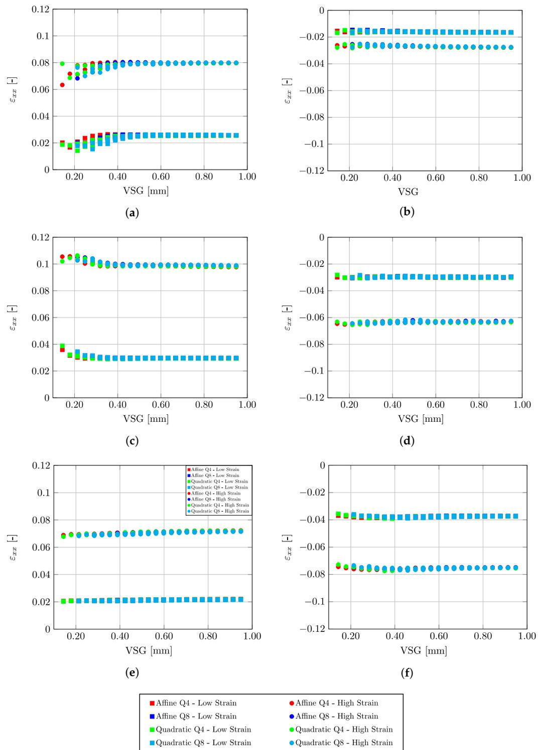
**Figure 4.** Evaluation of  $\epsilon_{xx}$  for points A, B, and C (Figure 3) as a function of DIC parameters expressed with regard to Virtual Strain Gauge (VSG) for both tension and compression tests, at two stages of deformation corresponding low and high strains. (a) Point A—Tension; (b) Point A—Compression; (c) Point B—Tension; (d) Point B—Compression; (e) Point C—Tension; (f) Point C—Compression.
