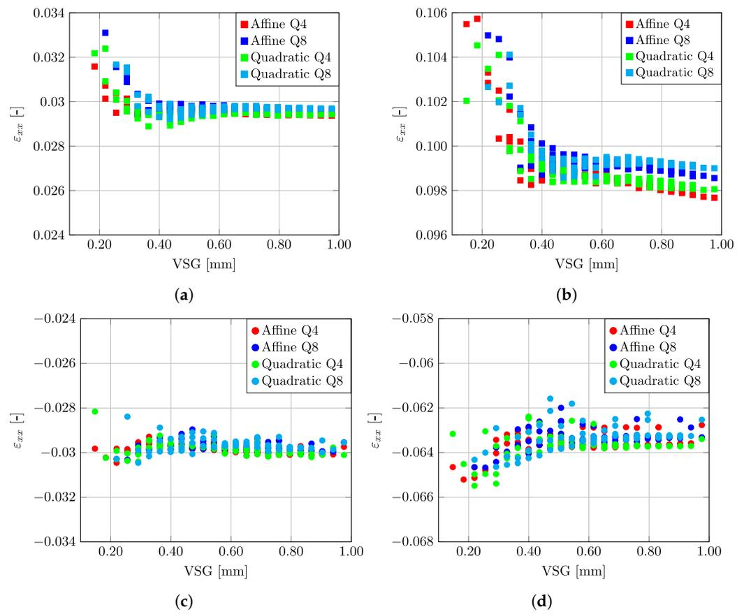
**Figure 5.** Evaluation of  $\epsilon_{xx}$  at point B (Figure 3) as a function of DIC parameters expressed with regard to Virtual Strain Gauge (VSG). (a) Tension-Low Strain; (b) Tension—High Strain; (c) Compression—Low Strain; (d) Compression—High Strain.
