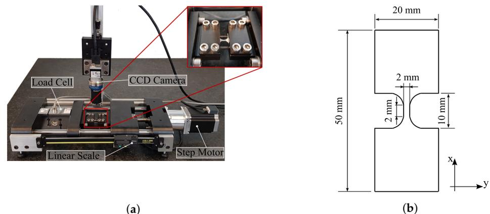
**Figure 2.** Miniaturized Specimen Tester Device (MSTD): (a) setup, and; (b) geometry of the miniaturized specimen.
