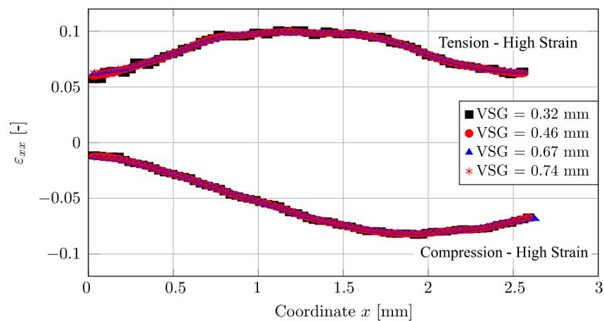
**Figure 6.** Evaluation of  $\epsilon_{xx}$  as a function of the coordinate  $x$  for several Virtual Strain Gauge (VMSG) values for both tension and compression tests.
