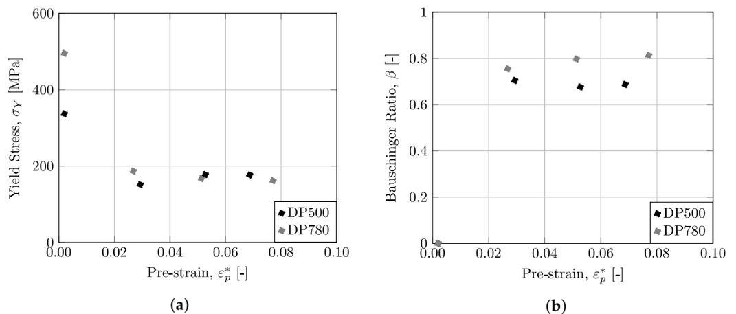
Figure 11. (a) Yield stress,  $\sigma_Y$ , and (b) Bauschinger Ratio,  $\beta$ , values for different pre-strains,  $\epsilon_p^*$ .
