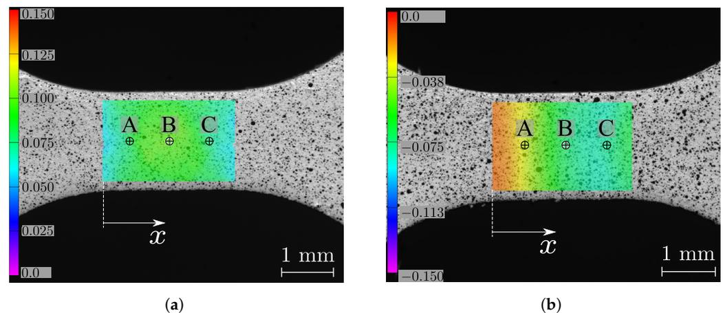
**Figure 3.** Points of reference used in evaluating the reconstruction of the  $\varepsilon_{xx}$  strain signal with regard to the DIC settings and as a function of the VSG for both (a) tension and (b) compression tests.
