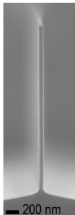
**Figure 10.** A GaAs nanowaveguide structure after passivation layer has been removed with an aspect ratio of  $>32$ , with a  $\text{N}_2$  flux of 11.8% ([115], used with permission from the Copyright Center and the contact author).
