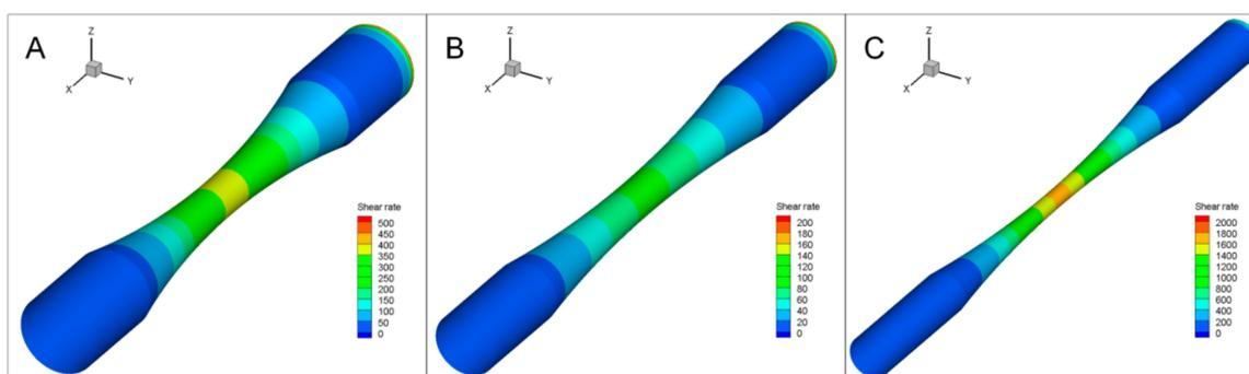
**Figure 8.** Computational simulation of wall shear rates (WSRs) in microchannels with a stenotic shape: Computational fluid dynamics analysis displayed WSR within the channel bottom in a microchannel. (A–C) Templates' inner diameters were  $390\text{ }\mu\text{m}$ ,  $330\text{ }\mu\text{m}$ , and  $125\text{ }\mu\text{m}$ , respectively, and the stenosis percentage ranged from 67.2% to 84.5%.
