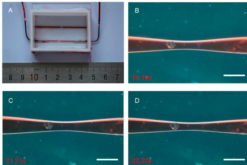
**Figure 2.** The microchip and liquid transport properties of artificial blood vessel: (A) The microchip perfused with oil red O, showing the liquid transport properties of the microchannel. (B–D) The original (B), expanded (C), and contracted (D) status of the microchannel. Scale bar, 100  $\mu\text{m}$ .
