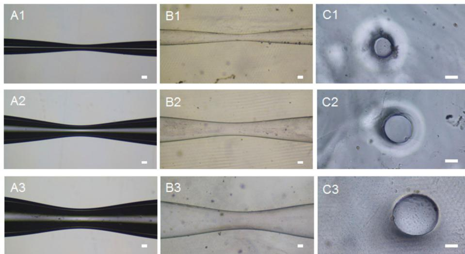
**Figure 1.** The tapered capillary tubes and engineered microchannels: (A1–A3) Photographs of the tapered capillary tubes; (B1–B3) Photographs of the gelatin chip with microchannels after removing the capillary templates and perfused with distilled water; (C1–C3) Cross-sectional view of the microchannels at the narrowest point. Scale bar, 100  $\mu\text{m}$ .
