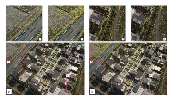
**Figure 11.** The influence of geometric rectification on feature extraction in terms of distribution and feature number: (**a**) feature detection on the original image; (**b**) feature detection on the rectified image; and four sub-images labeled with 1, 2, 3 and 4 are listed in the first row.
