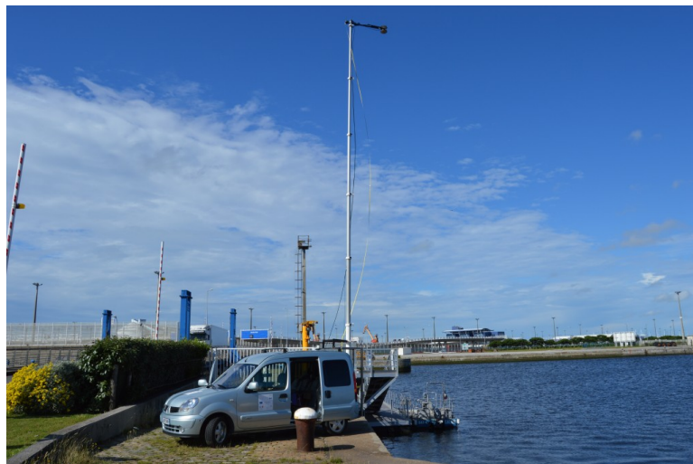
Figure 8. Experimental vehicle carrying the GNSS-R altimeter. The observed GPS signals are reflected on an artificial basin in Calais, France (50.962689°N, 1.857305°E).
