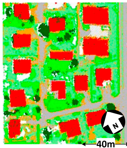
Figure 13. Generated land cover map (classification result). Six classes are coded by colors (red = “building”, light green = “grass”, dark green = “tree”, green = “hedge and bush”, grey = “road and parking lot”, orange = “wall and car port”). Taken from [12].
