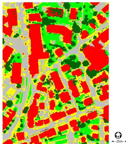
Figure 9. Classification result (red = “building”, dark green = “tree”, green = “low vegetation”, grey = “impervious surface”, yellow = “car”, blue = “clutter”).
