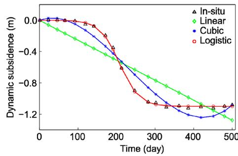
**Figure 10.** Comparison of the fitted dynamic subsidence using the linear, cubic polynomial, and logistic models.
