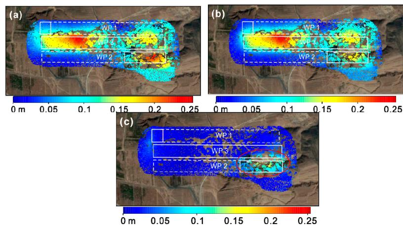
**Figure 9.** (a–c) Fitting residuals between the 17 InSAR observation maps and the synchronous ones estimated by the linear model, the cubic polynomial model, and the logistic model.
