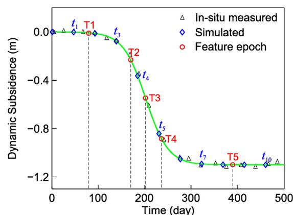
**Figure 2.** Simulated dynamic subsidence at a ground surface point.
