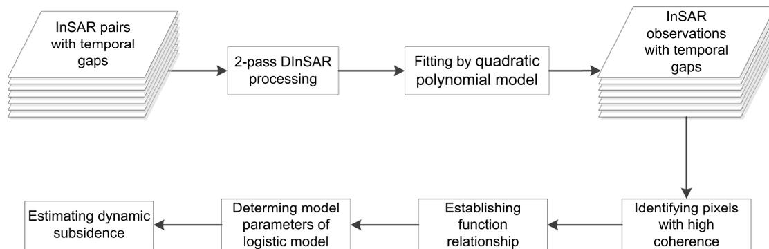
**Figure 1.** Block diagram of deriving dynamic subsidence of coal mining areas from InSAR observations with temporal gaps.
