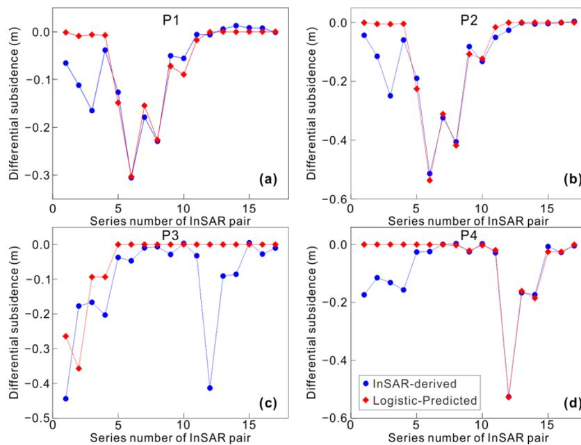
**Figure 11.** Comparison between the differential subsidence obtained by the InSAR-derived observations and the logistic-estimated synchronous results at points P1 to P4 (their locations are marked by the red points in Figure 8), respectively in (a–d).
