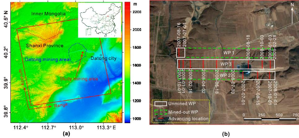
**Figure 4.** (a) Geographic location of the Datong mining area and the coverage of the SAR acquisitions superposed on the topographic relief shade map. (b) Advancing locations of the working panels from 1 July 2007 to 28 February 2009, overlain on the optical image acquired on 8 March 2014. The green dashed and white solid rectangles denote the mined-out and unworked working panels.
