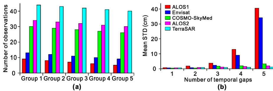
**Figure 3.** (a) Number of simulated InSAR observations with different numbers of temporal gaps, where Groups 1–5 contain 1–5 temporal gaps, respectively. (b) Mean STDs of the differences between the simulated dynamic subsidence and the subsidence estimated from the InSAR observations with temporal gaps using the proposed method.
