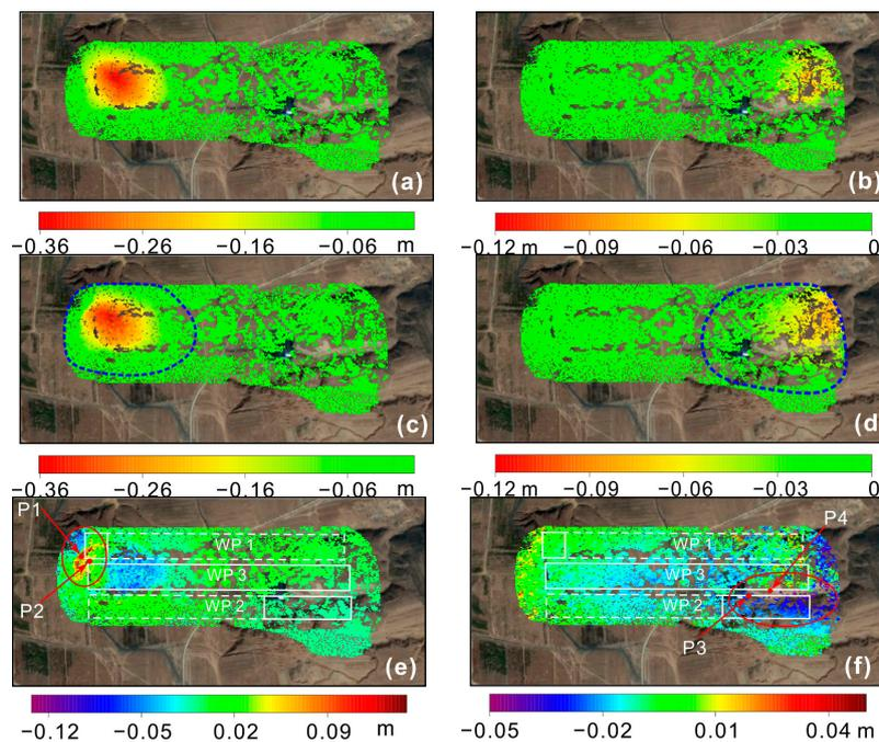
**Figure 8.** (a,b) InSAR-derived subsidence from 15 December 2007 to 30 January 2008 and from 16 September to 17 December 2008. (c,d) Logistic model derived synchronous subsidence. (e,f) Differences between the two sets of results. The red points in (e) and (f) are selected for further analysis.
