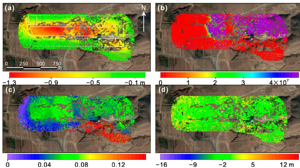
**Figure 6.** (a–c) Estimated model parameters  $W_0$ ,  $a$  and  $b$  of the logistic model; (d) Estimated topographic errors.
