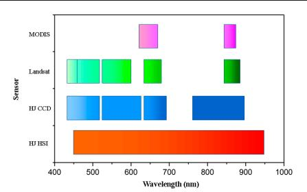
**Figure 3.** The spectral distributions of HSI (115 bands) versus CCD, Landsat 8 and MODIS in the 400–1000-nm range. Each color means one type of sensor, and each block means one band of the corresponding sensor.
