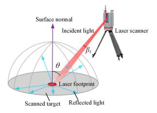
**Figure 1.** Reflected light of a laser footprint on a perfect diffuse target is uniformly scattered into a hemisphere.
