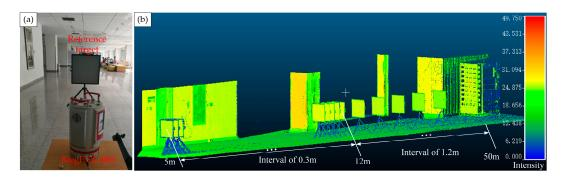
**Figure 4.** Experimental setup and scene of the distance experiment. (**a**) experimental setup including Riegl VZ-400i and three reference targets with reflectance of 15%, 30% and 60%, respectively; (**b**) scene of the distance experiment with distance from 5 m to 50 m, and a step interval of 0.3 m from 5 m to 12 m, and 1.2 m from 12 m to 50 m, respectively.
