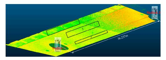
**Figure 5.** Point cloud of the multi-station scans colored with raw intensity data. (Note that Nos. 1, 2 and 3 represent the paving brick, concrete road and marking line, respectively. The distance between the center of station 1 and station 2 is 36.237 m).
