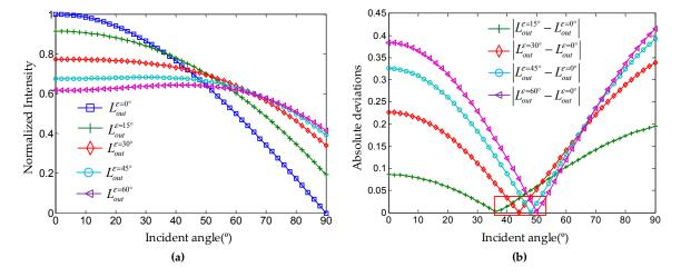
**Figure 8.** Simulated results of Oren–Nayar model vs. Lambert model. (a) normalized intensity data for different surface roughness parameters; (b) absolute deviations of  $L_{out}^{\varepsilon=15^\circ}$ ,  $L_{out}^{\varepsilon=30^\circ}$ ,  $L_{out}^{\varepsilon=45^\circ}$ ,  $L_{out}^{\varepsilon=60^\circ}$  from  $L_{out}^{\varepsilon=0^\circ}$ .
