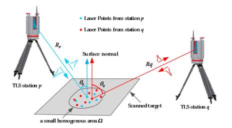
**Figure 3.** Schematic diagram of the proposed method to estimate the optimal value of the surface roughness parameter using the intensity data from TLS stations *p* and *q* in a small homogenous area  $\Omega$ .  $R_p$  and  $R_q$  are the distances from laser points to TLS stations *p* and *q*, respectively.  $\theta_p$  and  $\theta_q$  are the incident angles between the surface normal and the incident lights from TLS station *p* and *q*, respectively.
