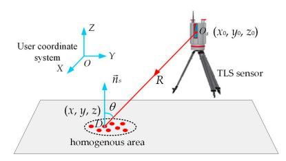
**Figure 2.** Geometrics of terrestrial laser scanning (TLS) for calculating the distance *R* and the incident angle  $\theta$ , where *O*-*XYZ* is the user coordinate system, the 3D coordinates of points *D* and *O*<sub>s</sub> are defined as (*x*, *y*, *z*) and (*x*<sub>0</sub>, *y*<sub>0</sub>, *z*<sub>0</sub>).
