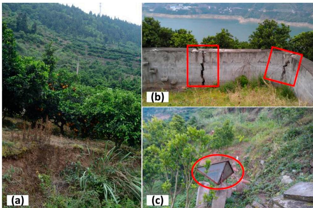
**Figure 2.** (a) Landscape of the landslide area; (b) Cracks on local infrastructure caused by the landslide; (c) one of the Corner Reflectors installed in the landslide area. Photos were taken during a field campaign in May 2014.
