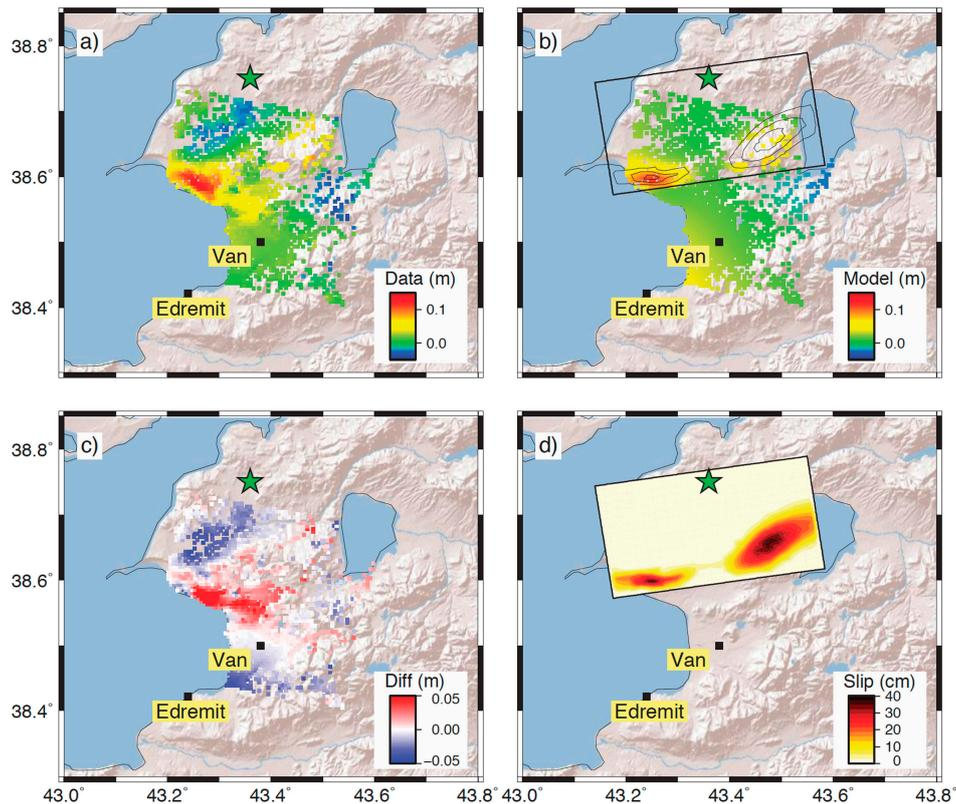
**Figure 10.** Post-seismic InSAR data and modeling (17-days temporal baseline): (a) subsampled data (step of 500 m, 1590 data points) computed from the difference between images CSK3 and TSX2 (see text for details); (b) modeled LOS displacements and the fault afterslip contour each 10 cm; (c) residuals (observed minus modeled data); and (d) related afterslip distribution. The green star is the mainshock epicenter.
