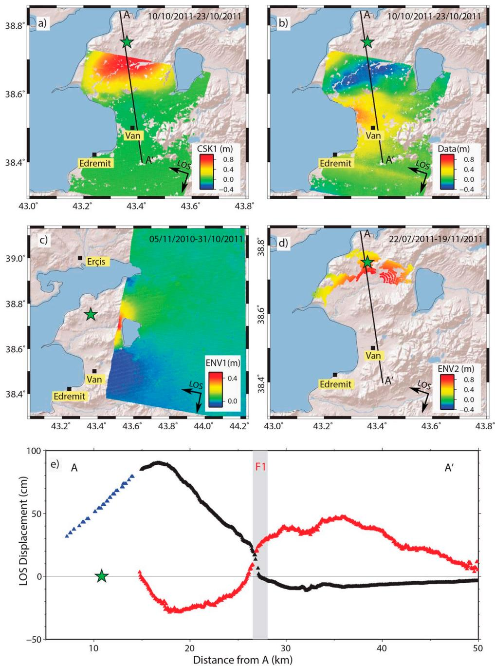
**Figure 3.** InSAR results: (a) CSK range results (*i.e.*, LOS direction); CSK1; (b) CSK azimuth results (positive Northwards); (c) ENV1, LOS displacements; and (d) ENV2, LOS displacements. SAR data details can be found in Table 1; (e) Data along the profile AA': CSK1 (range measurements, black), CSK (azimuth measurements, red), and ENV2 (LOS measurements, blue). The grey vertical band indicates the fault trace (F1) and its uncertainty (~1 km). The green star is the hypocenter.
