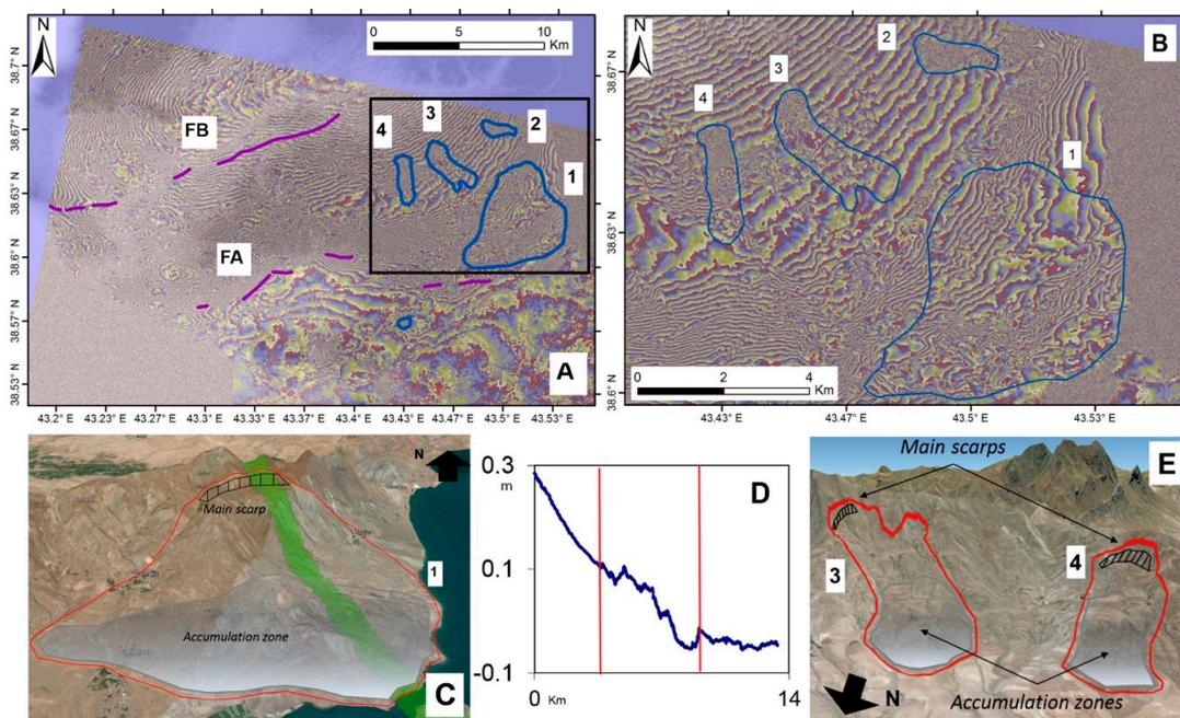
**Figure 4.** Fractures and landslides from InSAR: (A) wrapped phase of the CSK interferogram, where some crack lineaments (FA and FB, purple lines) and landslides (blue lines) are recognized; (B) zoomed view of the landslides; (C) Google Earth view from South of landslide 1 (red lines); and in green the displacement profile shown in (D), where the two red bars indicate the DGSD body; (E) Google Earth view from NNW of landslides 3 and 4, indicated in red.
