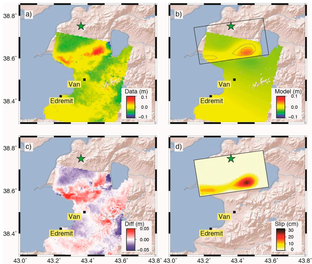
**Figure 9.** Post-seismic InSAR data and modeling (three-day temporal baseline): (a) subsampled CSK2 data (step of 500 m, 5660 data points); (b) modeled LOS displacements and the fault afterslip contour each 10 cm; (c) residuals (observed minus modeled data); and (d) related afterslip distribution. The green star is the mainshock epicenter.
