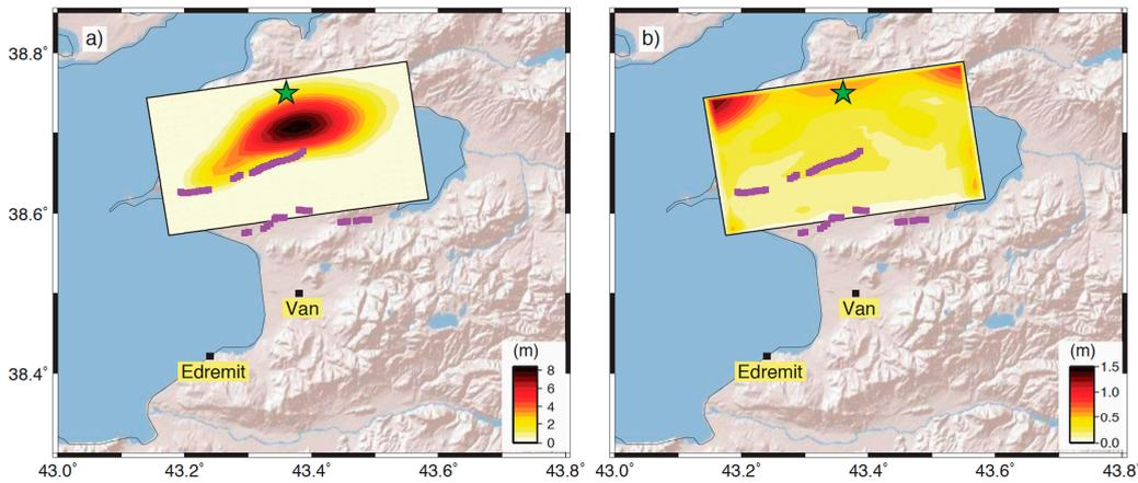
**Figure 6.** Fault slip distribution retrieved from geodetic data: (a) fault slip distribution; and (b) error associated. The surface fractures are reported by purple lines, and the Van earthquake epicenter by the green star.
