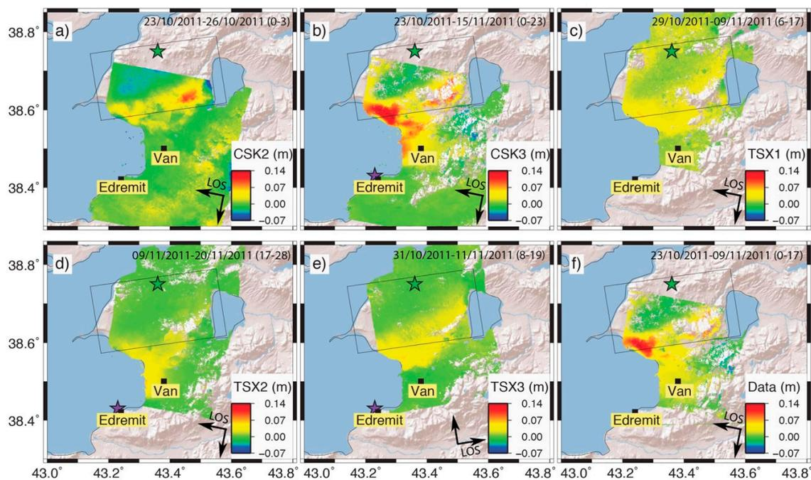
**Figure 8.** Post-seismic InSAR results from CSK and TSX satellites: (a) CSK2; (b) CSK3; (c) TSX1; (d) TSX2; (e) TSX3; and (f) difference between CSK3 and TSX2 (see text and Table 1 for details). Master/slave dates are indicated, along with the days after the mainshock in brackets. The green star is the mainshock epicenter and the purple star is the Edremit-Van earthquake epicenter (shown only if included in the temporal baseline).
