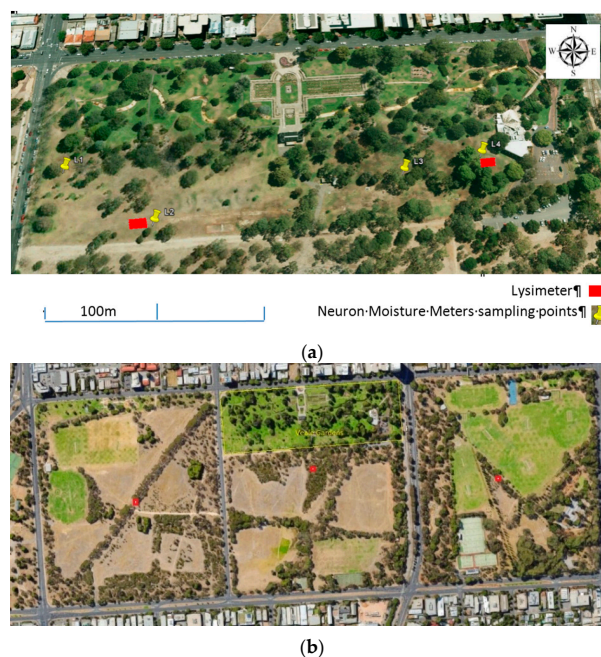
Figure 1. (a): instrument array for determining the soil/water balance in Veale Gardens (34,569.9140 S, 1,383,549.4899 E); (b): Lundie Garden, Veale Gardens, and Kurrangga Park, with red squares showing an approximate center of 250 m × 259 m. Resolution Imaging Spectroradiometer (MODIS) Enhanced Vegetation Index pixels obtained to determine evapotranspiration.2.2. Experimental Design.
