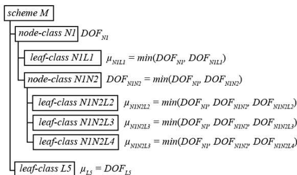
**Figure 1.** Hierarchical classification scheme with the *DOFs* of the *N*- and *L*-classes. Only *L*-classes have a membership degree  $\mu$ , expressed as the minimum of the *L*-class  $DOF_L$  and of its *N*-classes'  $DOF_N$ .
