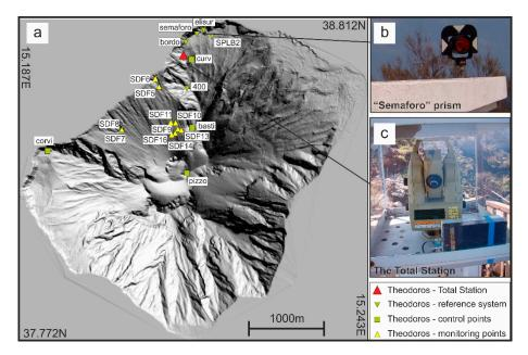
**Figure S1.** (a) Map showing the terrestrial robotized monitoring system of the *Sciara del Fuoco* (SdF) at Stromboli (THEODOROS); pictures on the right (b) show a typical reflecting prism and (c) the robotized Total Station.
