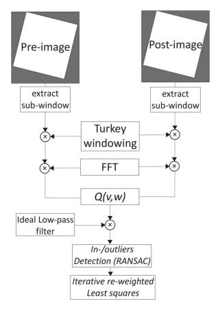
Figure S2. Algorithm workflow diagram of the applied robust phase fitting image cross-correlation method.
