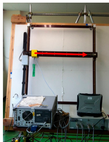
Figure 3. Developed polarimetric GB-SAR system. The line with an arrow indicates the position of the 1D survey line in Figure 1a.
