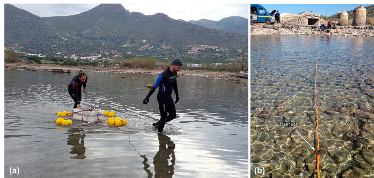
Figure 5. (a) Dynamic electrical resistivity tomography (ERT) data acquisition along individual lines forming a geophysical grid. The instrumentation was kept secure inside a custom made floating apparatus; (b) Cable used for the acquisition of static submerged ERT data.
