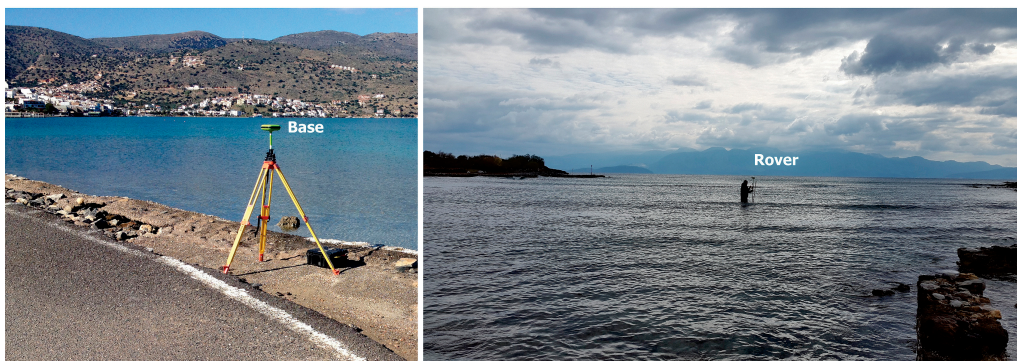
Figure 2. Base and rover Global Navigation Satellite System (GNSS) units used in the topographic mapping of Olous.
