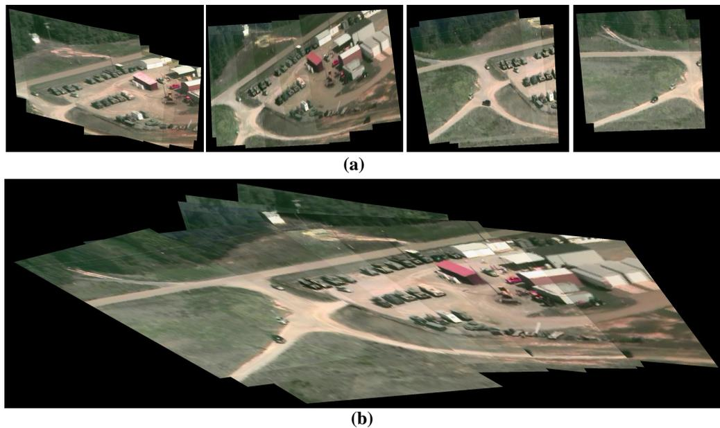
**Figure 3.** Example of sequential stitching vs. hybrid stitching. (a) Sequential stitching results over time with 4 panorama patches from 1 scene. (b) Our hybrid stitching result with a complete scene panorama
