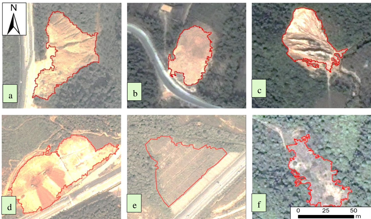
Figure 8. Examples showing the preparation of reference landslides in the case library, in the form of Quickbird images: (a–d) are young landslides (bright area with no vegetation cover); (e,f) are old landslides (less bright areas covered with concrete structures and vegetation).
