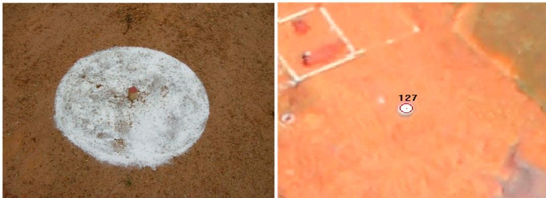
**Figure 4.** Layout of control points in Yangqiaodian and image positions of Ground Control Points.
