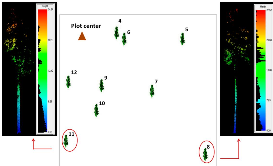
**Figure 11.** Reduction of the laser pulse penetration due to tree shadowing.
