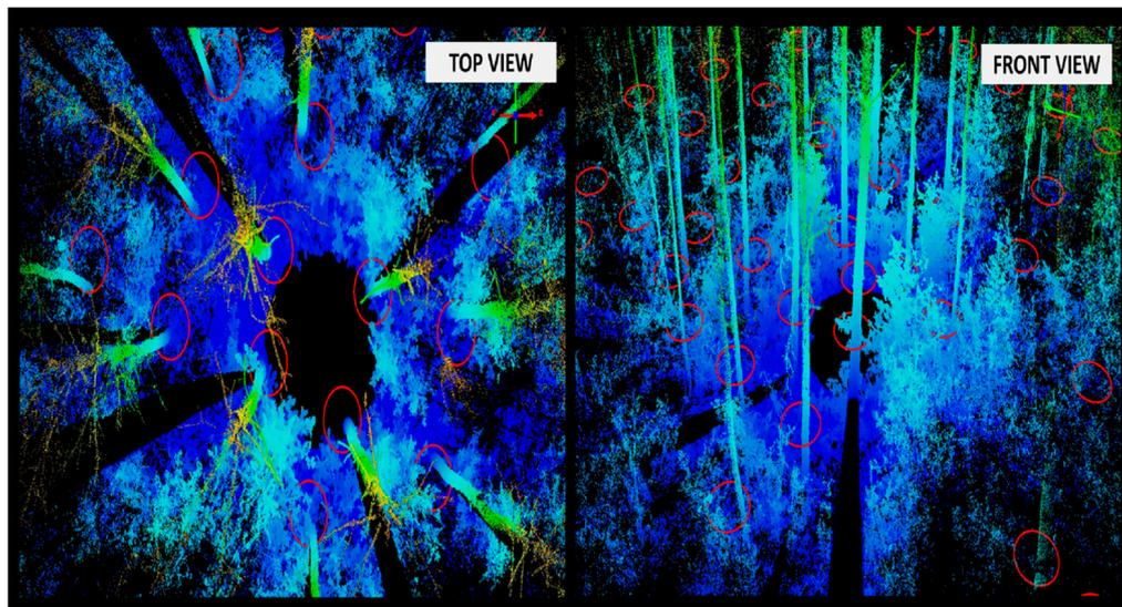
**Figure 4.** Mapped trees (represented in red circles) using distance and azimuth overlaid on the terrestrial laser scanning (TLS) point cloud for a 1/10th acre plot, site 2.
