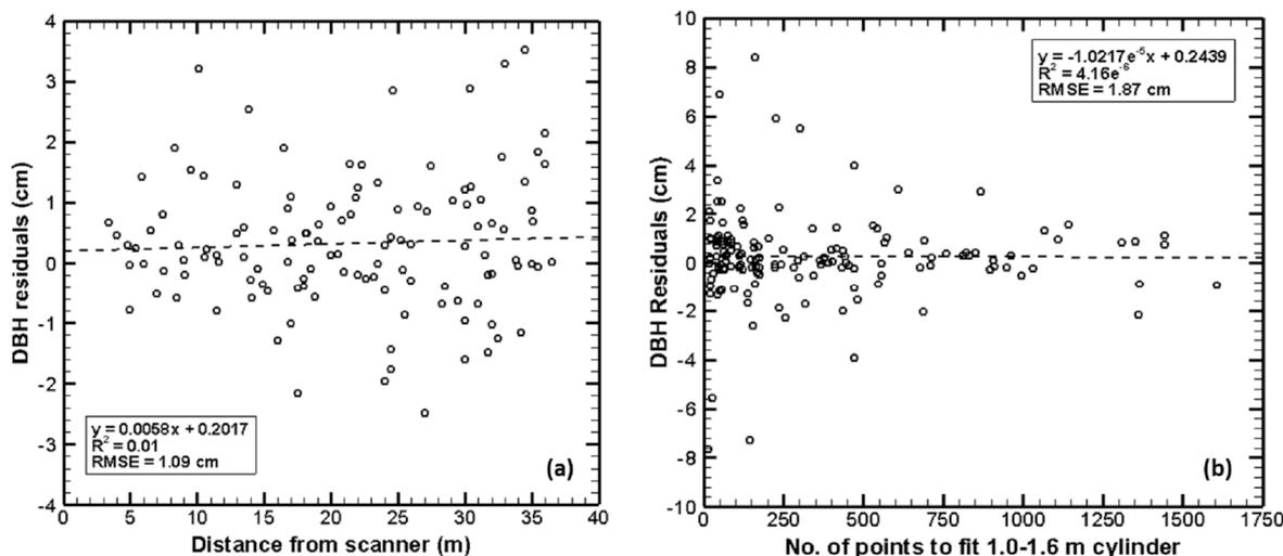
**Figure 8.** Diameter at breast height (DBH) residuals as a function of (a) distance from scanner (b) number of points to fit the cylinder.
