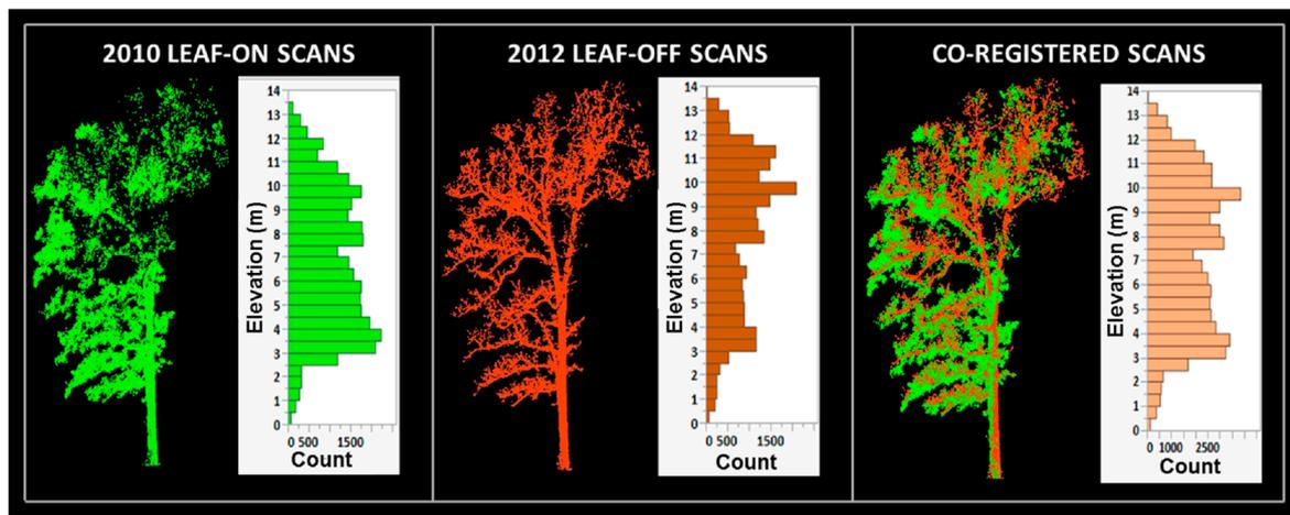
**Figure 3.** Co-registration of terrestrial laser scanning (TLS) scans for a post oak tree at site 1.
