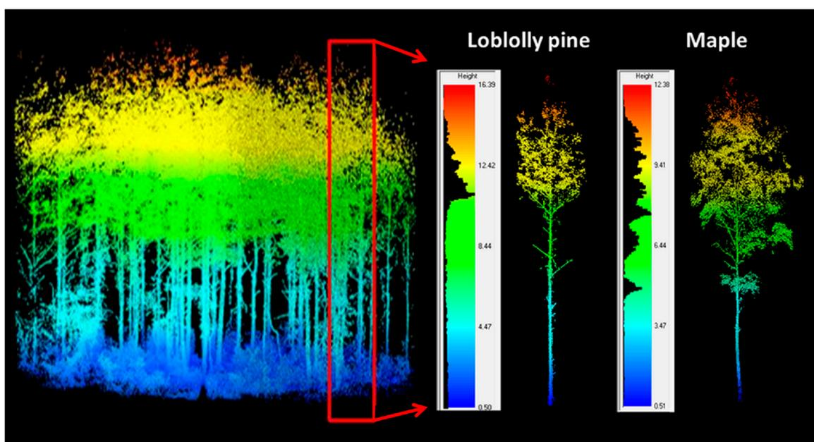
**Figure 6.** Extraction of individual trees using crown widths predicted from terrestrial laser scanning (TLS) derived diameter at breast height (DBH).
