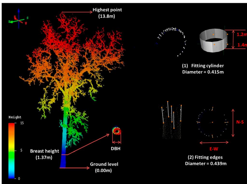
**Figure 5.** Diameter at breast height (DBH) retrieval methods by fitting cylinders and fitting edges on the terrestrial laser scanning (TLS) data.
