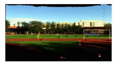
Figure 6. The rectified result with boresight calibration (the 12 CGPs are marked on it).
