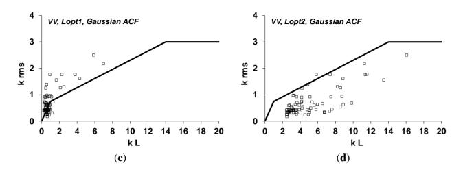
**Figure 4.** Validity regions of the IEM model in *k.rms* - *L* space (where *k* is the wave number) for Gaussian ACF, and the location of experimental data points [1]. All experimental data points are within the IEM limits with *Lopt2*. (**a**): HH polarization and *L*=*Lopt1*, (**b**): HH polarization and *L*=*Lopt2*, (**c**): VV polarization and *L*=*Lopt1*, (**d**): VV polarization and *L*=*Lopt2*.
