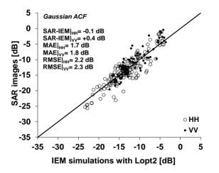
**Figure 8.** Validation of the semi-empirical calibration approach in using the fitting parameter *Lopt2*. Mean of the difference between SAR and IEM and root mean square error were calculated.
