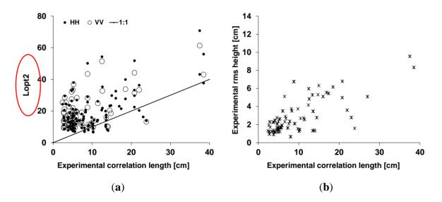
**Figure 6.** Relationship between (**a**) *Lopt2* with Gaussian ACF and the experimental correlation length; (**b**) the root mean square surface height and the experimental correlation length obtained from *in situ* measurements.
