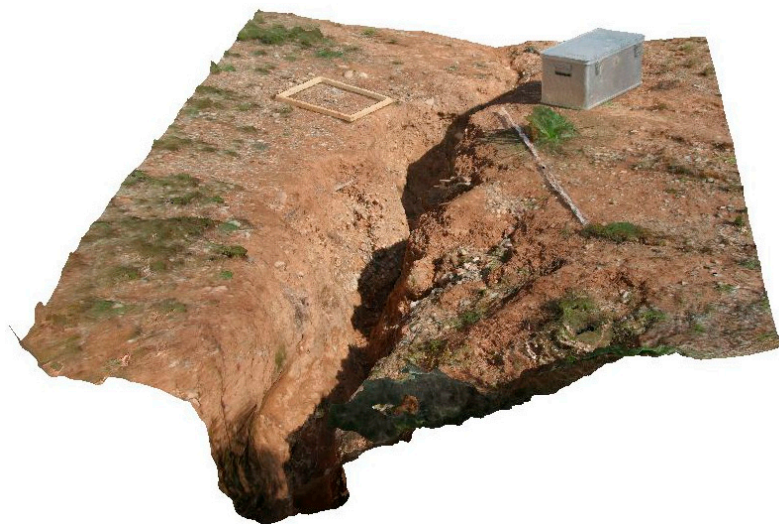
Figure 14. Final model with textures fitted onto the mesh of HAM in March 2013. Clearly visible are the scaling objects box, geometer (2 m) and wooden square ( 50 \times 50 \text{ cm}^2 ).
