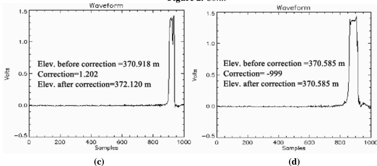
Figure 3. ICESat elevations across Lake Lemman extracted from the 3 June 2005 transect. The reference elevation is 372.18 m. Ordinate = energy in volts and abscissa = bin number (bin spacing = 1 ns).
