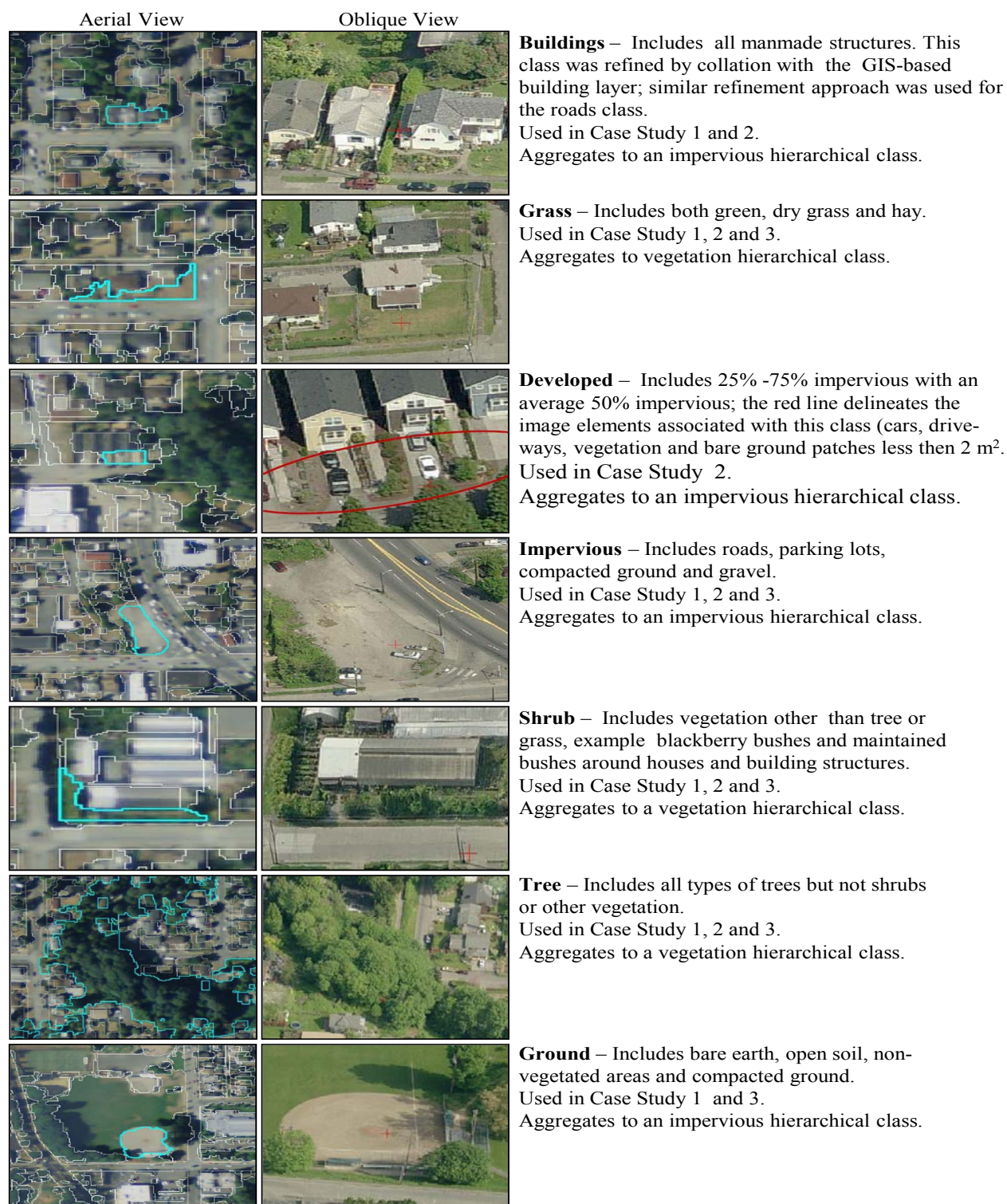
Figure 2. Example of image segments representative of the described LULC classes. Cyan polygons show an example of the LULC class being delineated in the OBIA segmentation, adjacent segments are shown in white and can represent a different class. The oblique image is centered on the delineated segment. The 2002 aerial and co-registered 2009 oblique images are not shown at the same scale; north is up.
