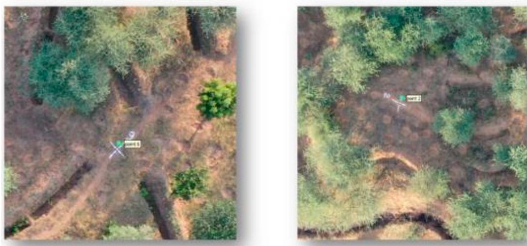
Figure 3. UAV aerial image showing marking of ground control points with number.
