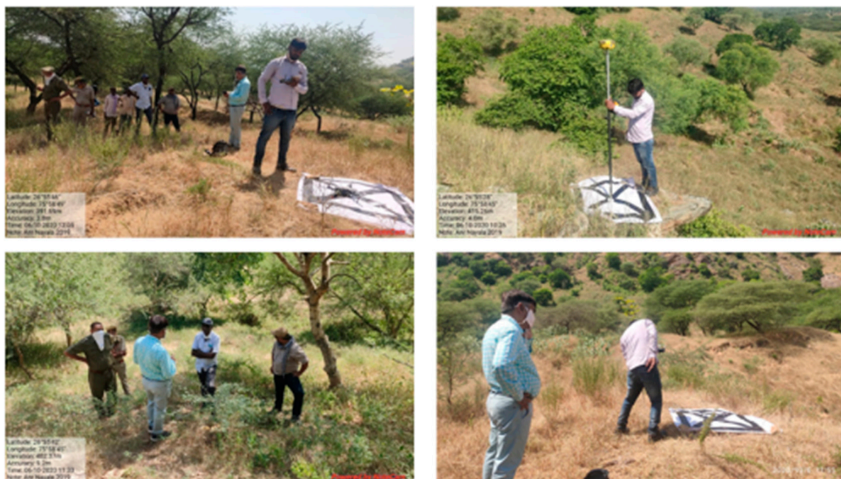
Figure 4. Field photographs showing field-based discussion. DGPS measurement on printed GCP.
