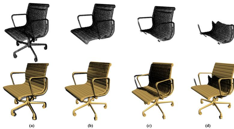
**Figure 12.** Reconstruction results with different degrees of occlusion: (a) 0%; (b) 50%; (c) 75%; (d) 90%.
