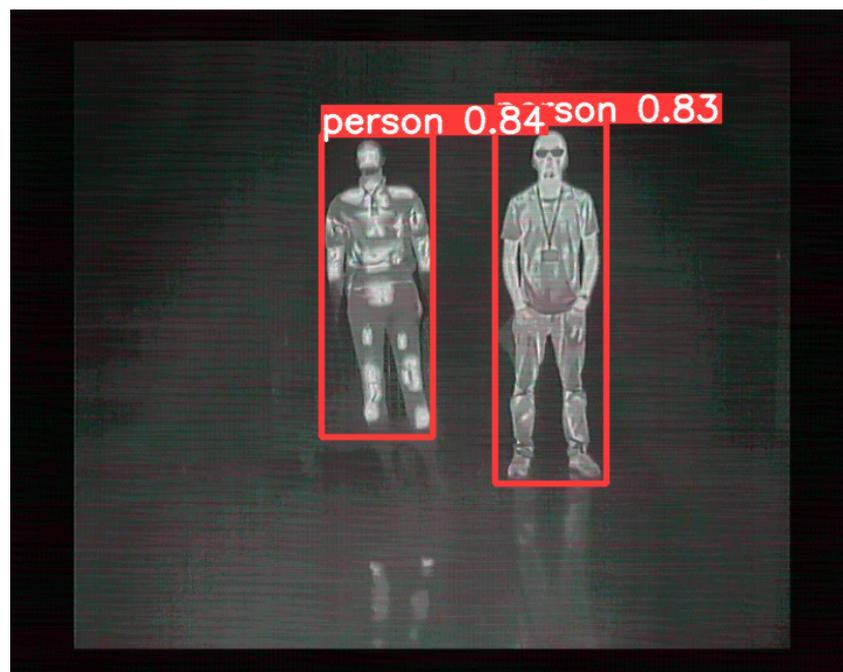
**Figure 15.** YOLOv5 detection output of thermal imagery with a heated mannequin and a human being.
