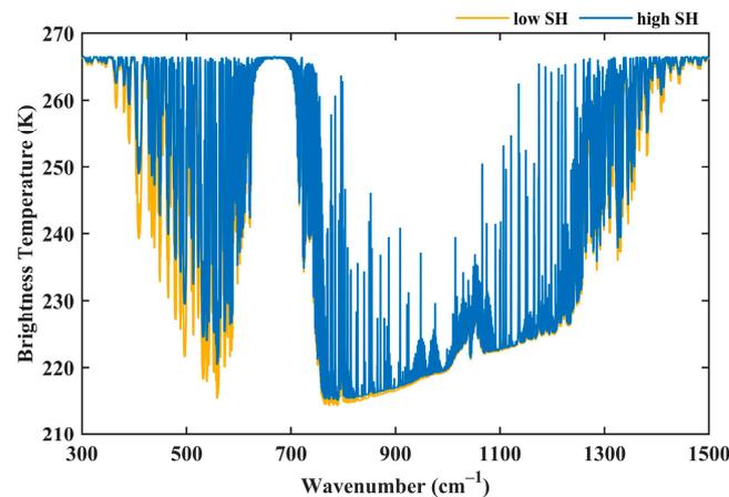
**Figure 2.** Hyperspectral brightness temperature simulations of ice clouds at different specific humidities (SH). The cloud optical depth ( $\tau$ ) is 1.0 and the effective radius ( $r_{eff,i}$ ) is  $30\ \mu\text{m}$ . The blue line indicates a high specific humidity, and the yellow line indicates a low one.
