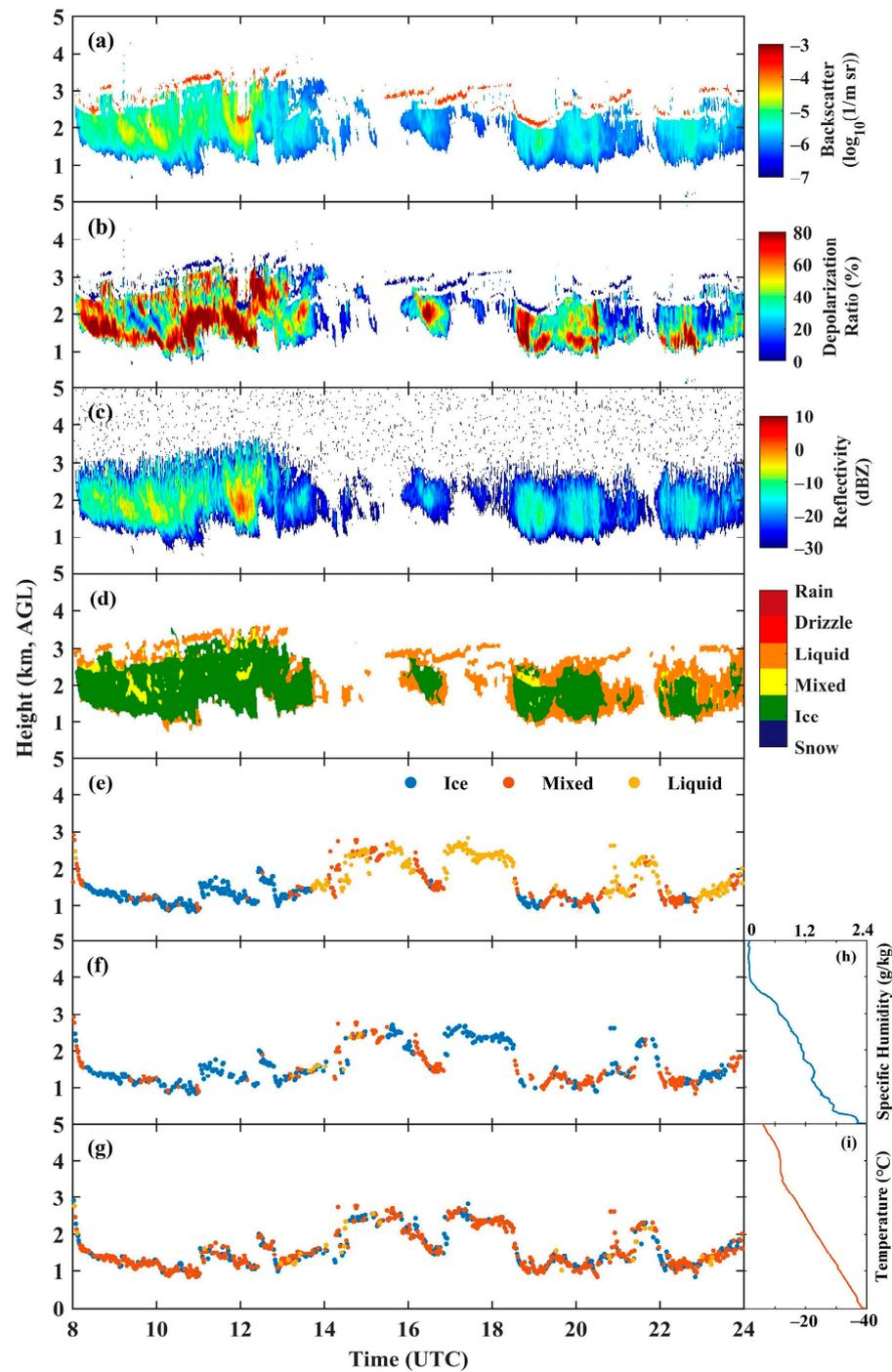
**Figure 8.** The (a) backscatter coefficient and (b) depolarization ratio from HSRL, the (c) reflectivity from KAZR, the (d) cloud phase profile using Shupe’s method, the cloud phase classification results of (e) Shupe’s, (f) Turner’s, and (g) the proposed methods, and the (h) average specific humidity and (i) temperature from 08:00 to 24:00 UTC on the 25 December 2016, in the AWARE. The results of the three methods are plotted at the clouds’ base heights using HSRL.
