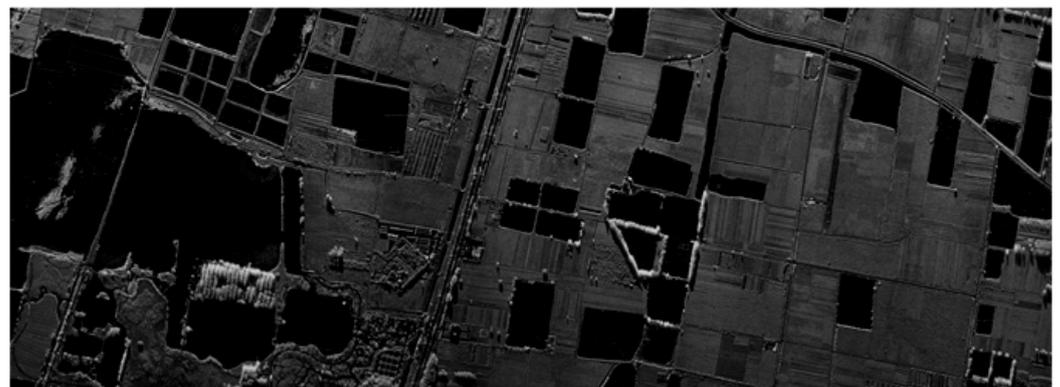
**Figure 5.** Real-time stripmap image of rural area at 0.3 m resolution.
