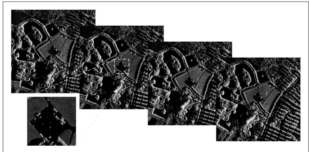
**Figure 6.** Real-time spotlight images of urban area at 0.15 m resolution.
