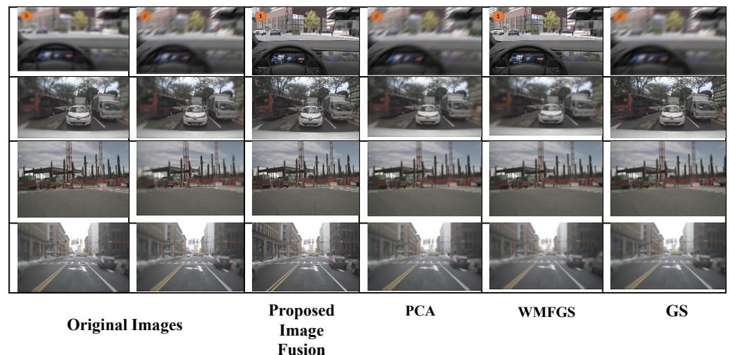
**Figure 15.** Performance comparison of different image fusion models. PCA-Principle Component Analysis, WMFGS-Weighed Mean Filter based Gram–Schmidt transform, GS-Gram–Schmidt transform.
