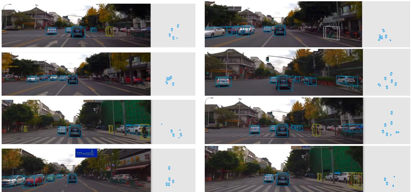
**Figure 11.** Real scenes application of the proposed Keypoint3D on the road of Chengdu, China. Cars, pedestrians, and cyclists are represented by pale blue, brown, and gray boxes, respectively. The heading direction is represented with a cross mark.
