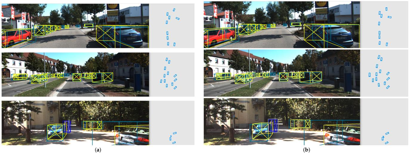
**Figure 9.** Qualitative comparisons of the detection performance in 3D and BEV on the KITTI *val* set. (a) Baseline work (CenterNet). (b) The proposed method (Keypoint3D). Ground truth labels present cars, pedestrians, and cyclists with yellow, red and blue boxes, respectively. The predicted results present cars, pedestrians, and cyclists with pale blue, brown, and gray boxes, respectively. The heading direction is represented with a cross mark.
