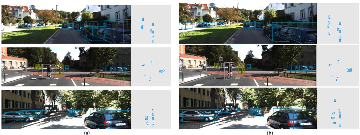
**Figure 10.** Qualitative comparisons of the detection performance in 3D and BEV on the KITTI test set. (a) Baseline work (CenterNet). (b) The proposed method (Keypoint3D). Cars, pedestrians, and cyclists are represented by pale blue, brown, and gray boxes, respectively. The heading direction is represented with a cross mark.
