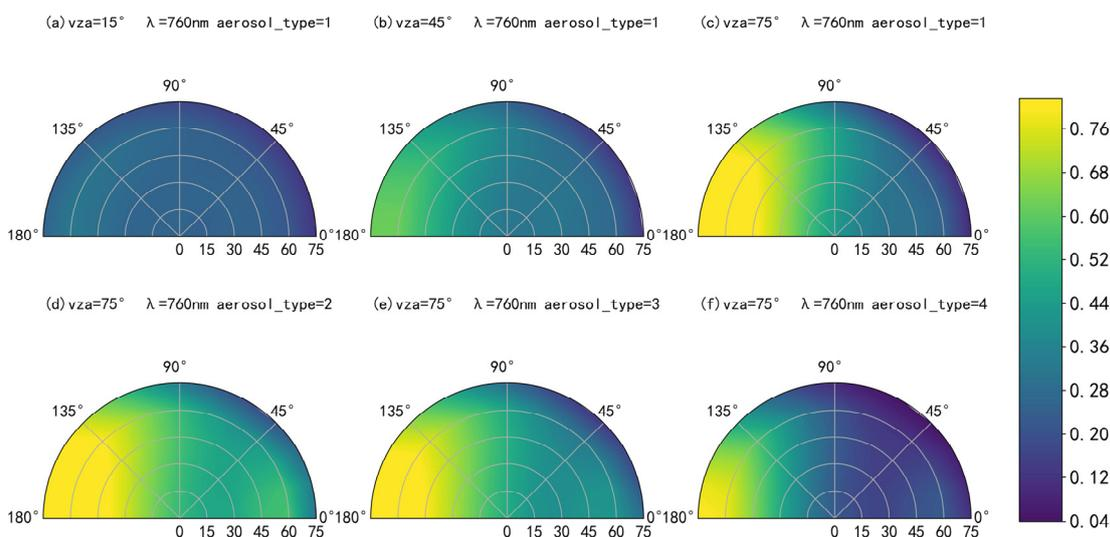
**Figure 3.** DFS of aerosol vertical profiles for different geometry: (a–c) VZA =  $15^\circ$ ,  $45^\circ$ ,  $75^\circ$  and (c–f) DFS of different aerosol vertical profiles for identical geometry.
