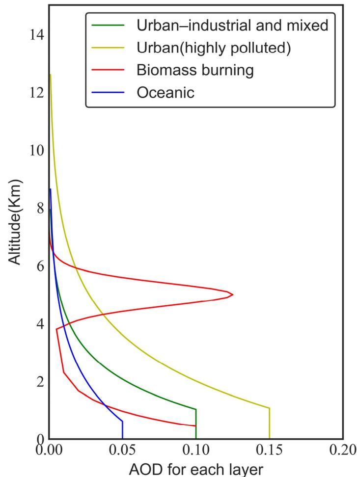
**Figure 1.** The four aerosol vertical profiles.
