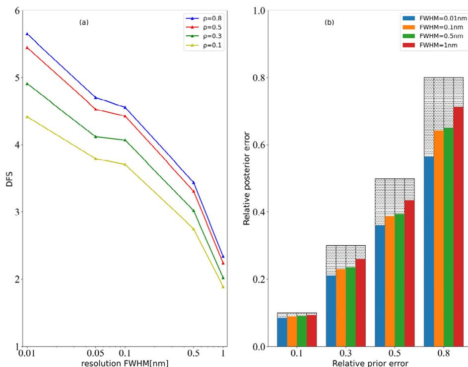
**Figure 8.** Influence of the prior error of aerosol vertical profiles for different spectral resolutions of urban-industrial and mixed aerosols: (a) influence on DFS values; (b) influence on posterior error.
