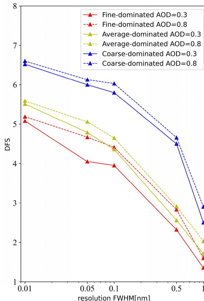
**Figure 7.** The influence of three aerosol size distributions on DFS value at different spectral resolutions.
