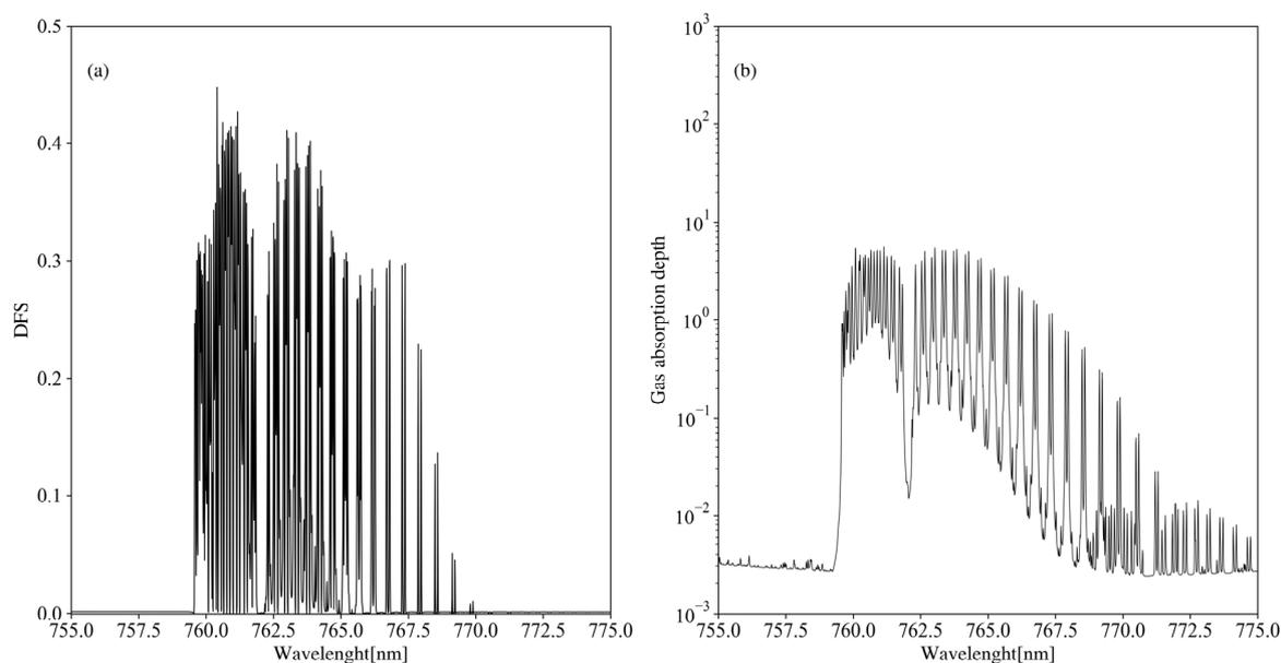
**Figure 2.** (a) DFS of individual channels in  $O_2$  A-band (b) Spectral absorption optical depth of atmosphere in the  $O_2$  A-band.
