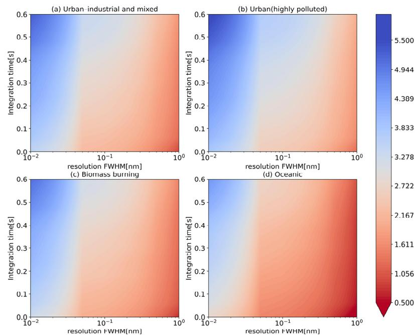
**Figure 5.** Influence of spectral resolution and integration time on DFS values of four aerosol vertical profiles.
