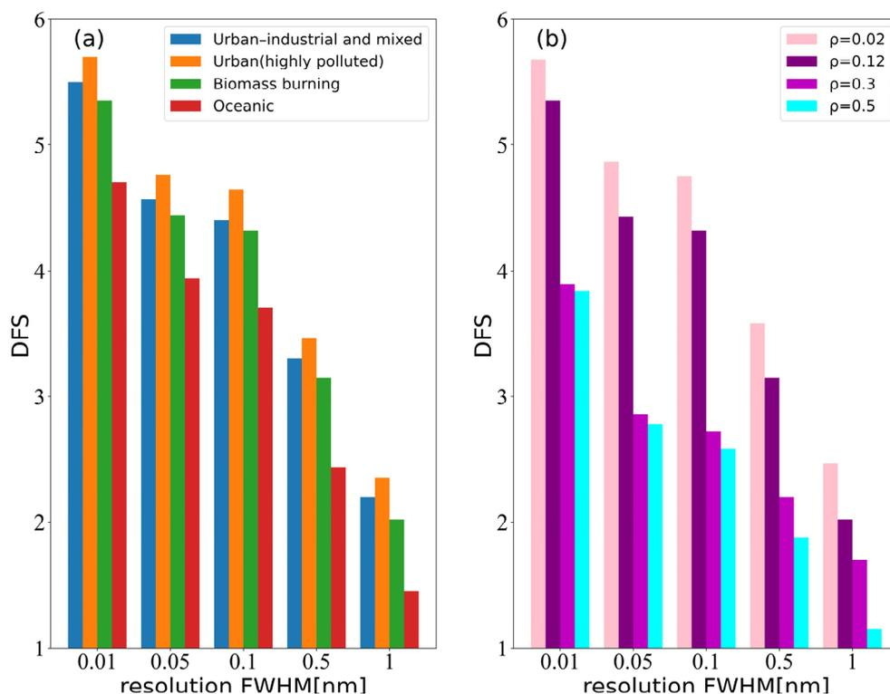
**Figure 4.** Influence of spectral resolution on DFS value: (a) DFS of four aerosol vertical profiles for different spectral resolutions; (b) DFS of biomass burning aerosol for different spectral resolutions and ground surface reflectivity.
