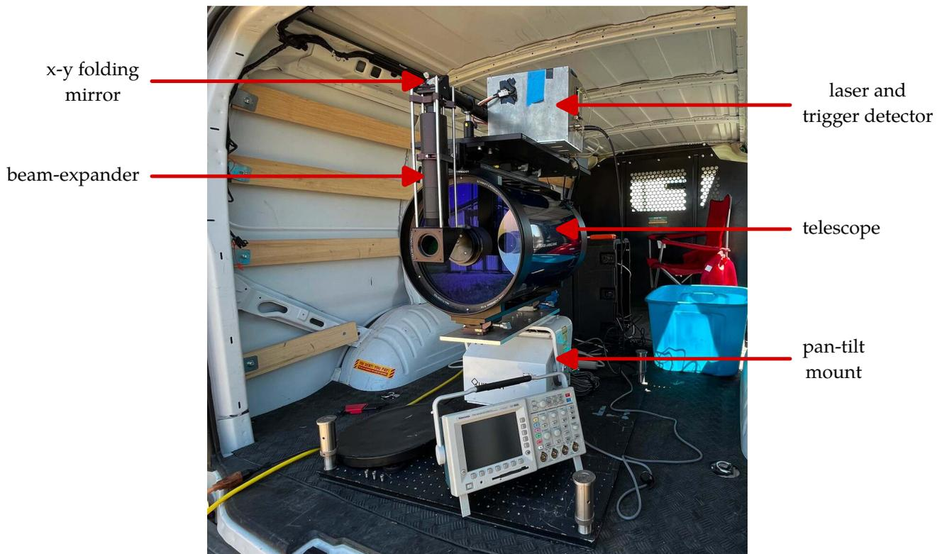
Figure 3. Picture of the lidar system during data collection.
