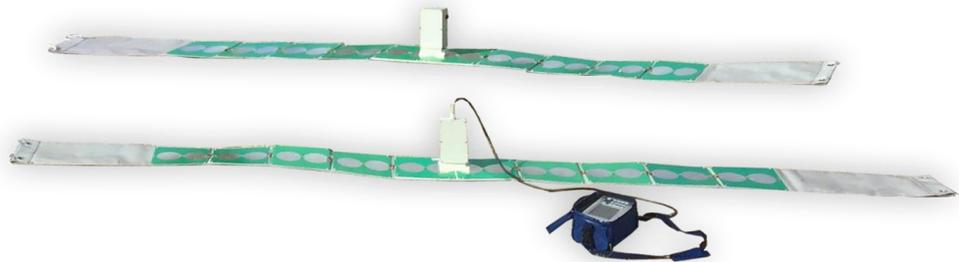
**Figure 2.** Loza-N GPR with 50 MHz (3 m long) antennas.
