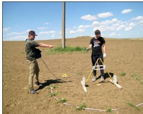
**Figure 6.** Measurements of GPR radiation pattern in the upper hemisphere under an electric power line.
