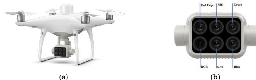
**Figure 6.** Unmanned aerial vehicles used for multi angle reflectivity measurement: (a) DJI P4M remote sensing system; (b) multispectral camera loaded on DJI P4M.
