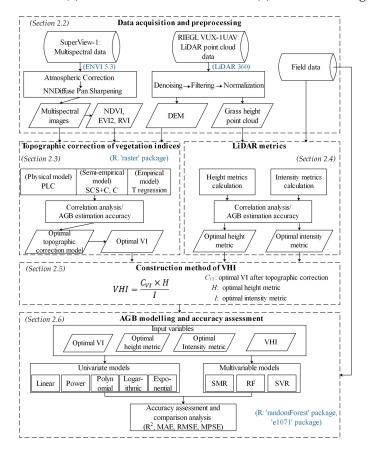
**Figure 1.** Flowchart of data processing and AGB estimation (The title of each step is highlighted in boldface. The main software used in the processing are highlighted in blue).
