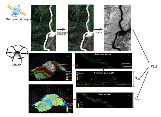
Figure 3. The workflow plot of the proposed VHI for biomass estimation.
