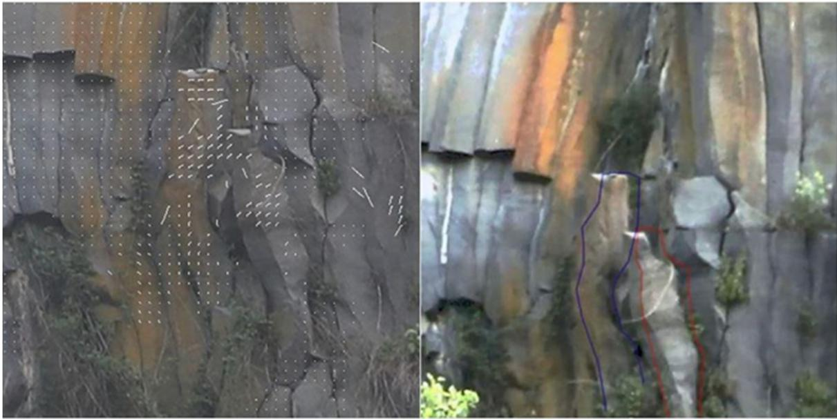
**Figure 8.** Left, movement vectors from camera 2. Right, in red and blue the original position of the columns.
