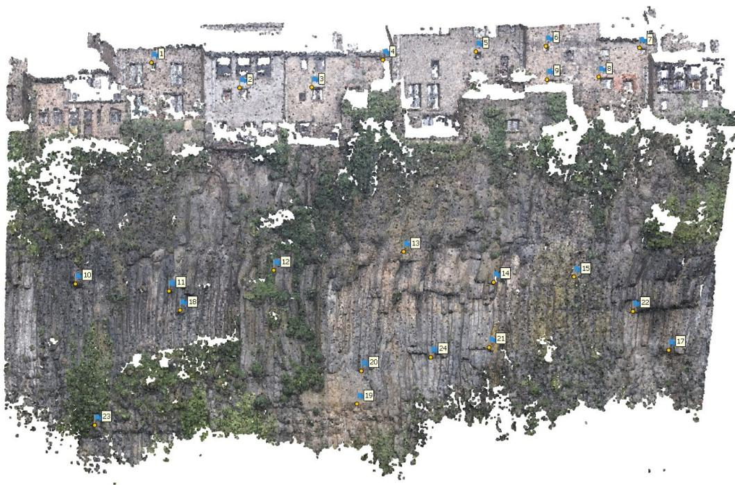
**Figure 6.** Photogrammetric model and distribution of control points.
