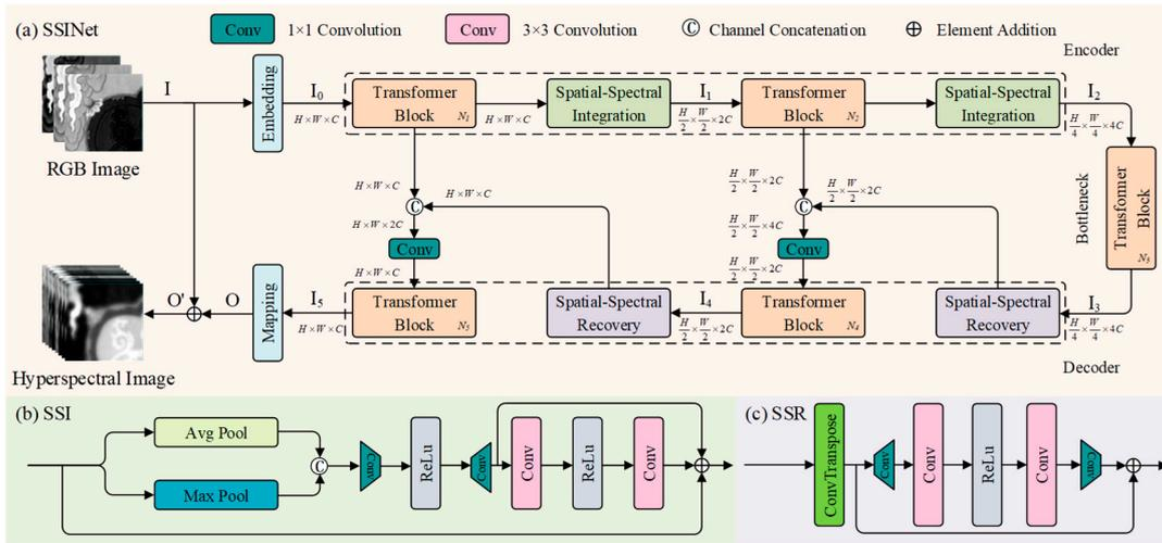
**Figure 1.** The general structure of SSINet, which consists of an encoder, a bottleneck, and a decoder, all of which feature multiscale hierarchical design with efficient Transformer blocks (a); (b) the components of Spatial–Spectral Integration (SSI); and (c) the components of Spatial–Spectral Recovery (SSR).
