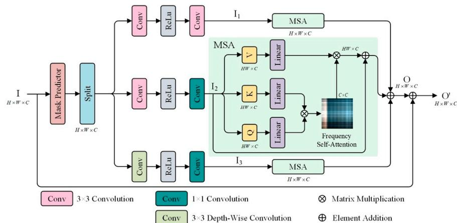
**Figure 2.** The essential modules of the Transformer block. The Mask Predictor determines the computation load of the frequency-wise branches, while F-MSA treats each computation load as a token and performs self-attention calculations along the spectral dimension.
