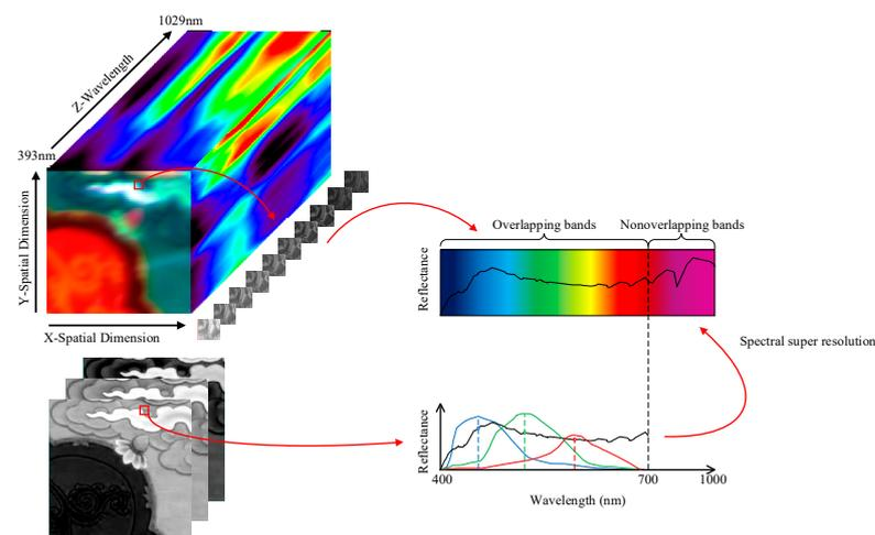
**Figure 4.** Diagram of RGB image generated (Canon 5DSR camera) and spectral reconstruction (RGB → Hyperspectral image).
