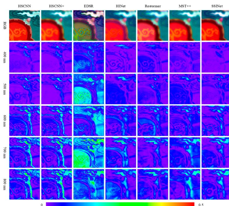
**Figure 5.** The first row displays the reconstructed RGB composition of HSI, while the remaining rows exhibit the visual results of the error map in the Thangka dataset.
