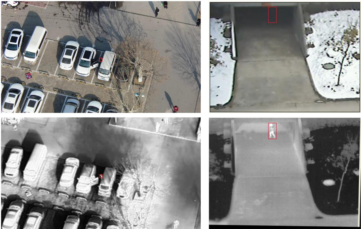
Figure 1. Examples where objects are tracked better in thermal infrared images (bottom).
