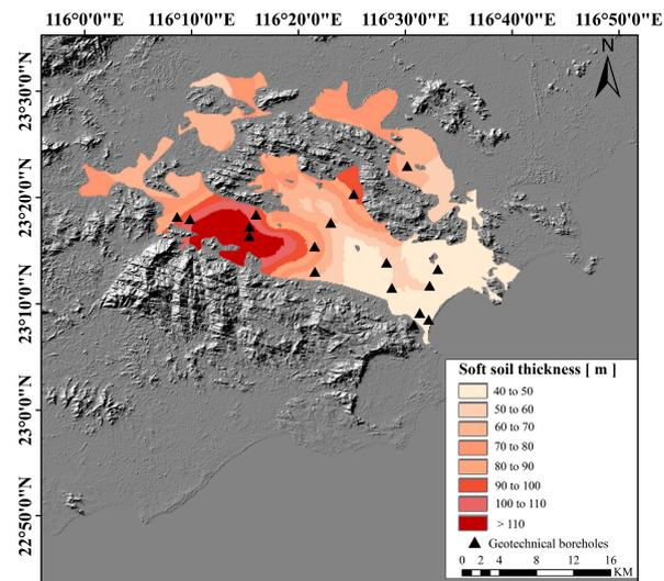
**Figure 2.** Sedimentary thickness map and borehole locations. The thickness of the sediment has been calculated by means of geotechnical borehole data.
