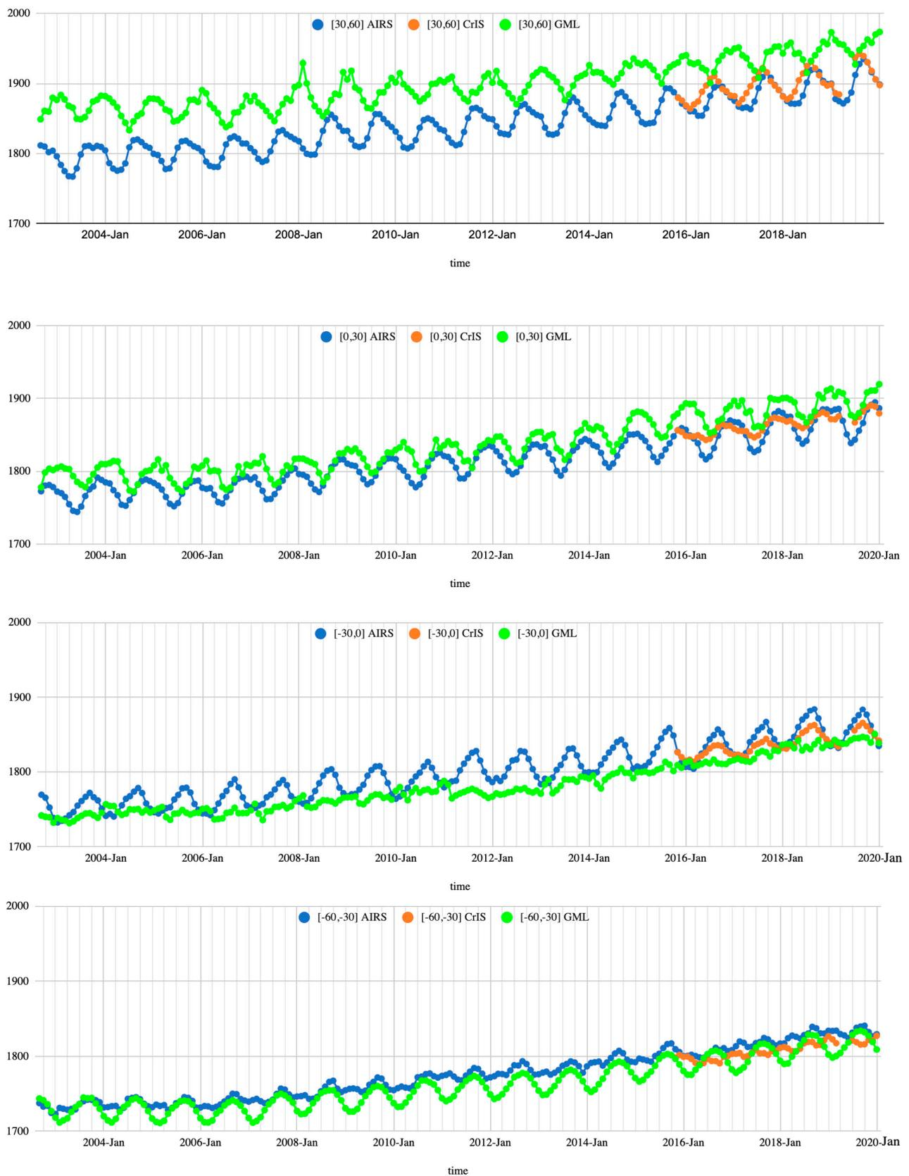
**Figure 5.** Time series of CH<sub>4</sub> (in ppb) retrieved from AIRS (blue), CrIS (orange) at 400 hPa, and in situ measurements from NOAA GML (green) for different latitudinal zones: 60–90°N (top panel); 30–60°N (2nd panel); 0–30°N (3rd panel); 0–30°S (4th panel); 30–60°S (lowest panel).
