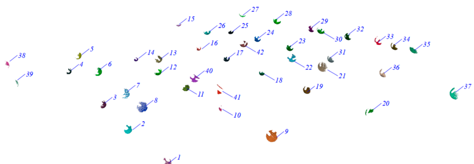
Figure 7. Sphere segmentation from large-scale PCD by VR-eSphere (different spheres are numbered and distinguished by colors).
