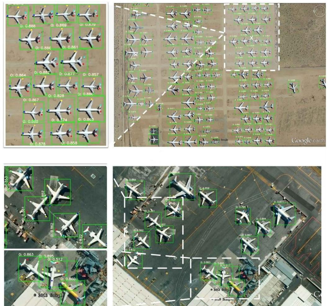
**Figure 8.** A more detailed visualization of the detection results at a higher resolution, showing that our method maintained its good performance with different backgrounds and obtained accurate landmarks.
