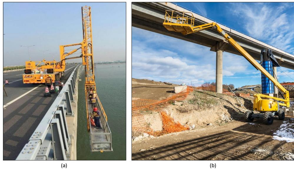
**Figure 1.** (a) Snooper Truck (Source: [5]. Reprinted with permission from Ref. [5]. Copyright 2021 MDPI); (b) Man Lift.
