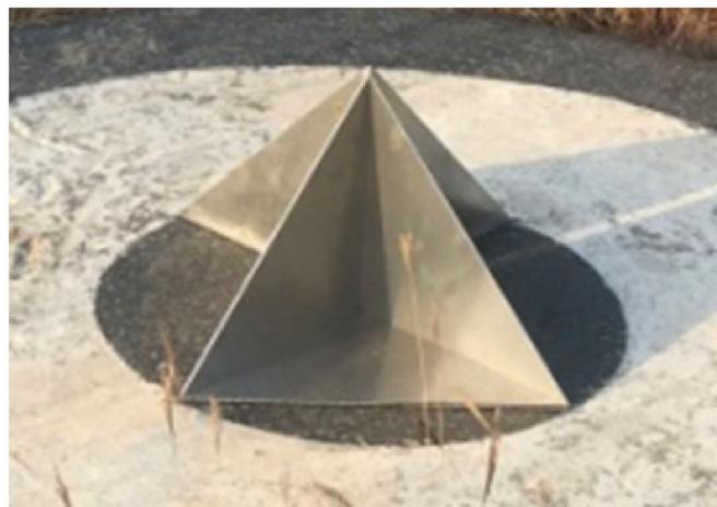
**Figure 2.** A metal corner reflector in the data acquisition experiments.
