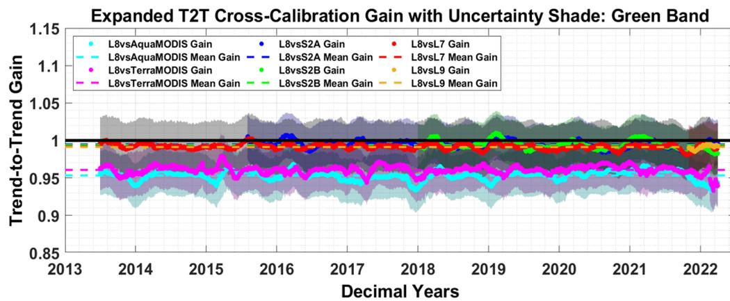
Figure 21. Expanded T2T cross-calibration gain of six sensor pairs for the green band using EPICS Global. The shaded region shows uncertainty associated with each pair of sensors.
