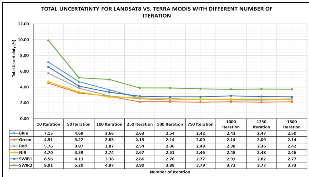
Figure 17. Total Uncertainty for Landsat 8 versus Terra MODIS with different numbers of iterations for all six bands using EPCIS Global.
