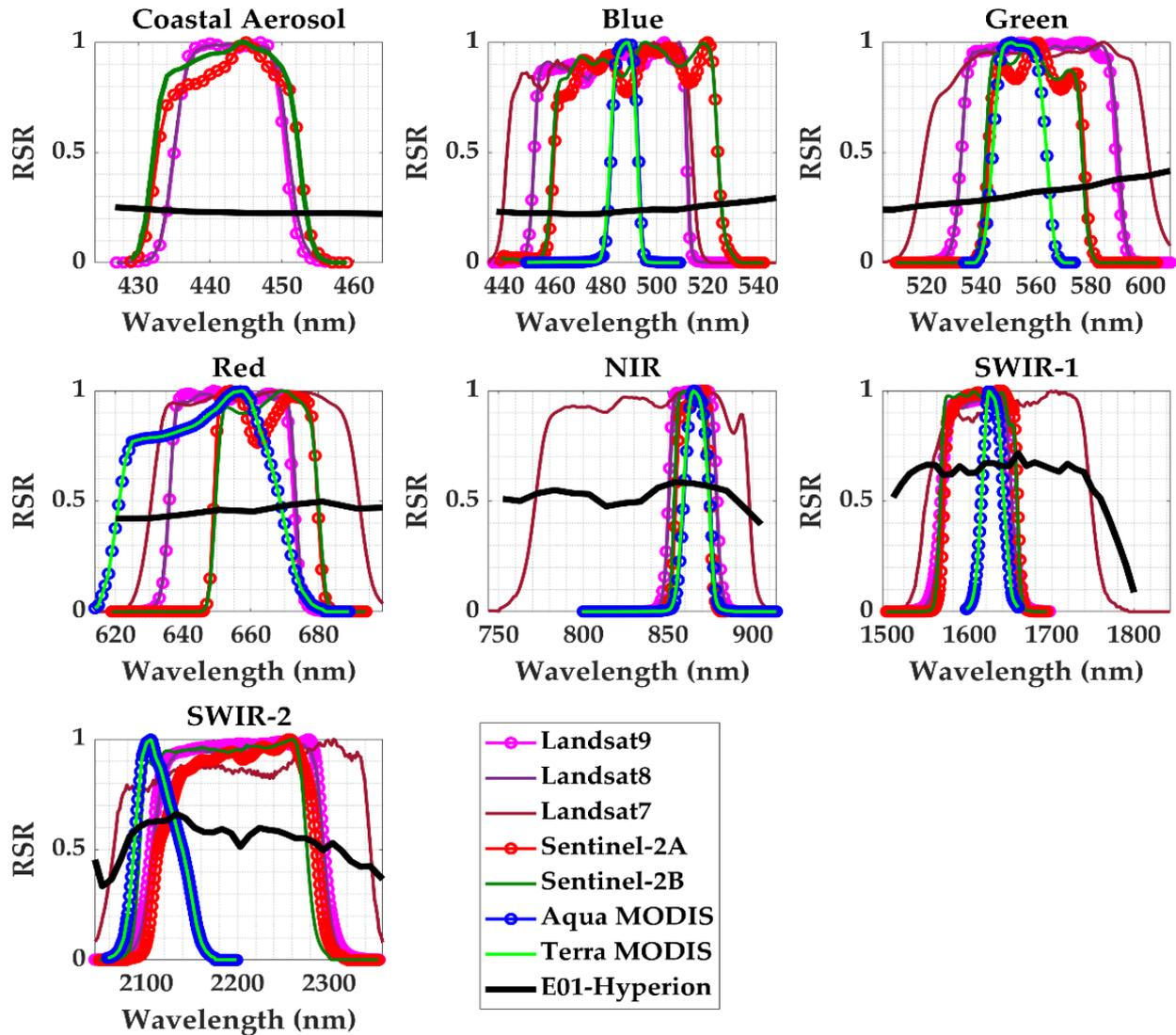
**Figure 9.** RSR of Landsat 9, Landsat 8, Landsat 7, Sentinel-2A, Sentinel-2B, Aqua MODIS, Terra MODIS, and the hyperspectral profile of Hyperion derived using EPICS Global.
