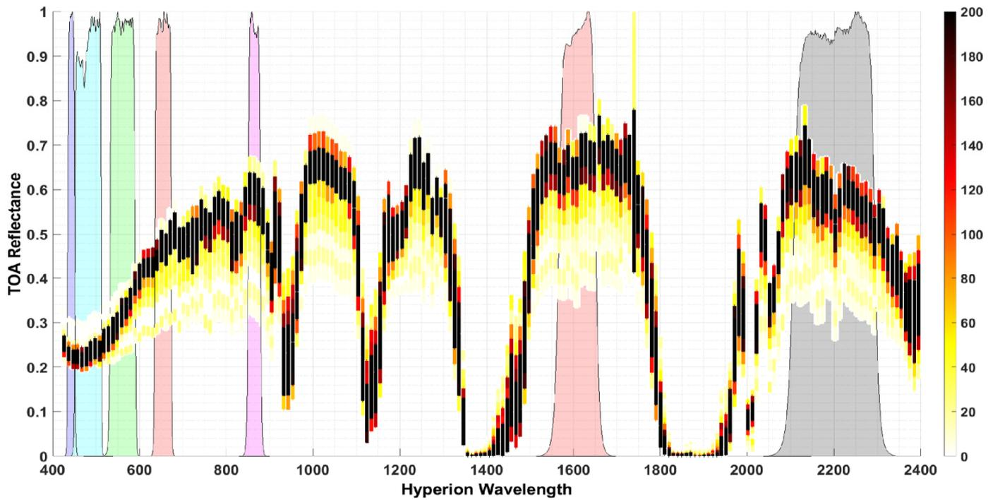
**Figure 3.** Hyperspectral profile of EPICS Global Data using Hyperion and shaded reason shows RSR for Landsat 8.
