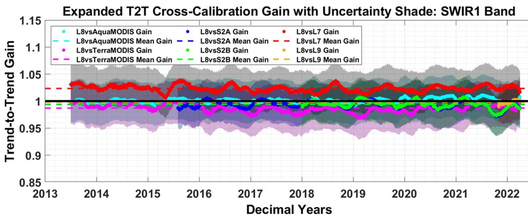
Figure 24. Expanded T2T cross-calibration gain of six sensor pairs for the SWIR1 band using EPICS Global. The shaded region shows uncertainty associated with each pair of sensors.
