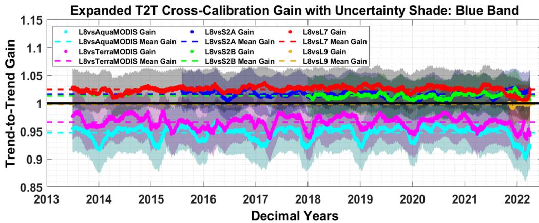
Figure 20. Expanded T2T cross-calibration gain of six sensor pairs for the blue band using EPICS Global. The shaded region shows uncertainty associated with each pair of sensors.
