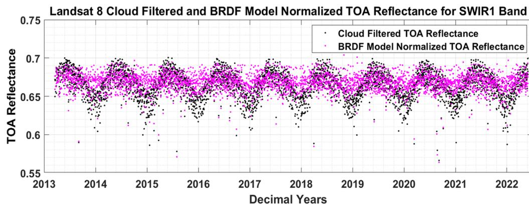
**Figure 13.** Black and magenta dots represent cloud-filtered TOA reflectance and BRDF normalized TOA reflectance of Landsat 8 for SWIR1 Band.
