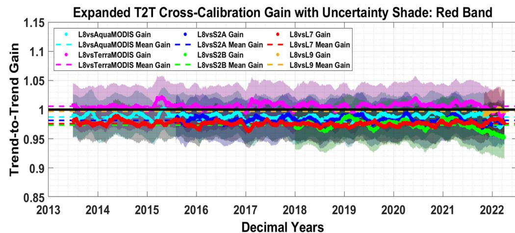
Figure 22. Expanded T2T cross-calibration gain of six sensor pairs for the red band using EPICS Global. The shaded region shows uncertainty associated with each pair of sensors.
