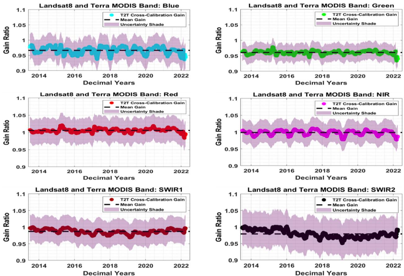
**Figure 18.** Trend-to-Trend Cross Calibration Gain with Mean Gain and Shaded region shows uncertainty associated with specific bands.
