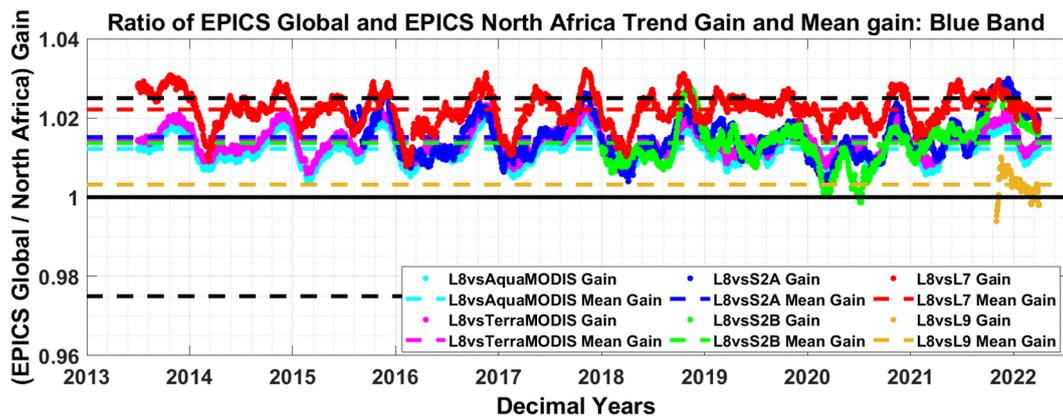
Figure 26. Ratio of EPICS Global and North Africa expanded T2T cross-calibration gain for six sensor pairs for the blue band.
