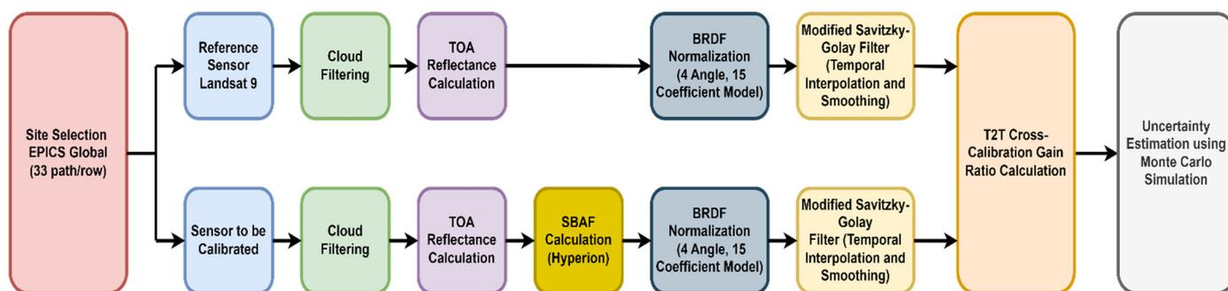
**Figure 1.** Workflow Diagram used for trend-to-trend Cross-calibration using Global EPICS.
