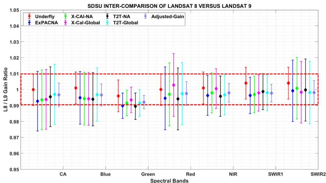
**Figure 7.** SDSU Inter-Comparison of Landsat 8 versus Landsat 9 results using four different techniques, and the red dotted box represents a 1% difference level.
