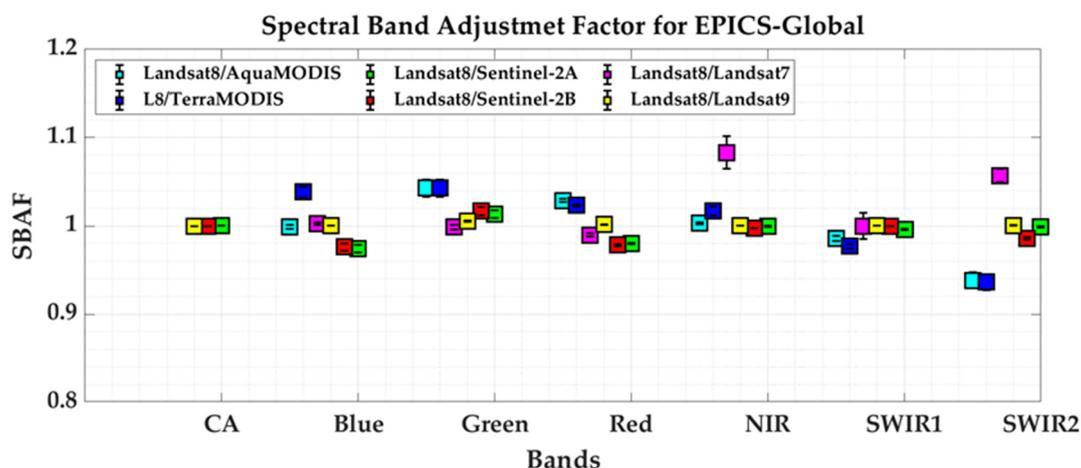
**Figure 10.** SBAF values calculated from the hyperspectral profile of Hyperion derived using Global EPICS for six pairs of sensors combination where Landsat 8 is as reference sensor, and denominator sensors are sensors needed to be calibrated. Error bars are the standard deviation ( $k = 2$ ).
