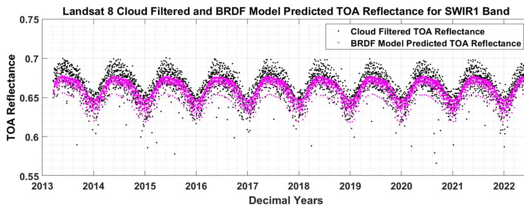
**Figure 12.** Black and magenta dots represent cloud-filtered TOA reflectance, and the BRDF model predicted the TOA reflectance of Landsat 8 for the SWIR1 Band.
