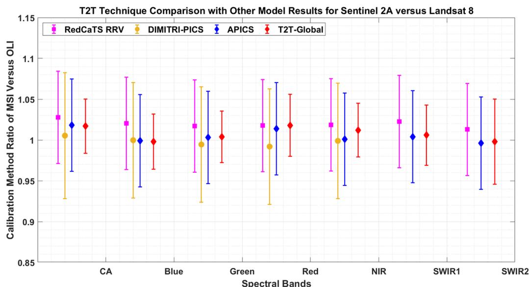
**Figure 6.** Trend-to-Trend Cross-Calibration result comparison with absolute calibration results for Sentinel 2A versus Landsat 8 and error bars for all models representing uncertainty. Two years of the dataset (2015–2017) for both sensors as initially used by Barsi.
