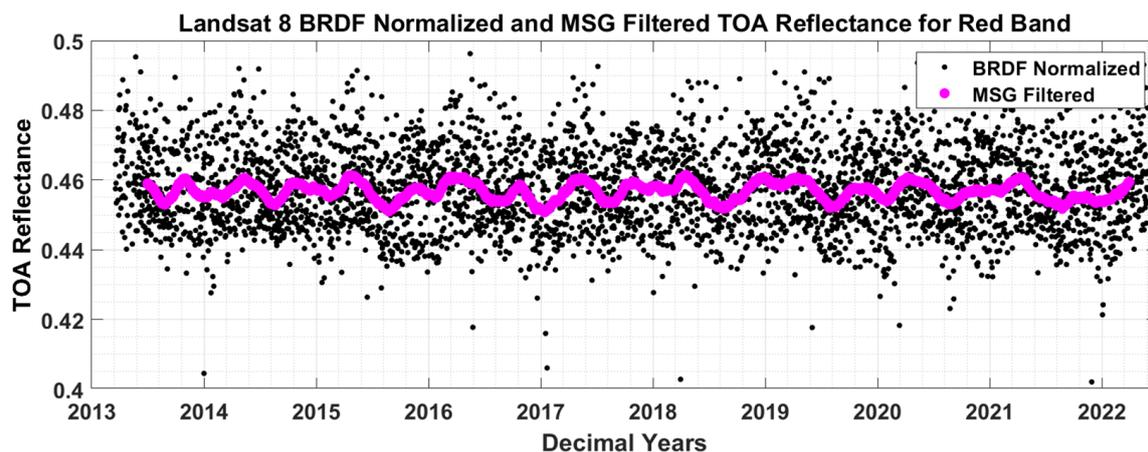
**Figure 15.** Black and magenta dots represent BRDF normalized TOA reflectance, and MSG filtered TOA reflectance of Landsat 8 for Red Band.
