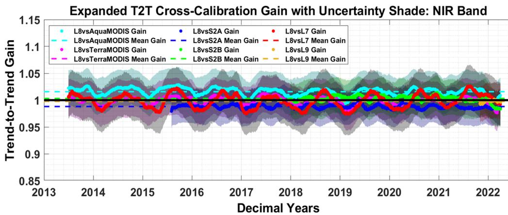
Figure 23. Expanded T2T cross-calibration gain of six sensor pairs for the NIR band using EPICS Global. The shaded region shows uncertainty associated with each pair of sensors.
