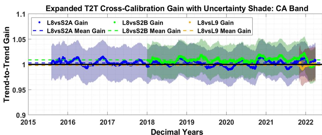
**Figure 19.** Expanded T2T cross-calibration gain of Landsat 8 versus Sentinel-2A/2B and Landsat 9 for coastal aerosol Band using EPICS Global. The shaded region shows uncertainty associated with each pair of sensors.
