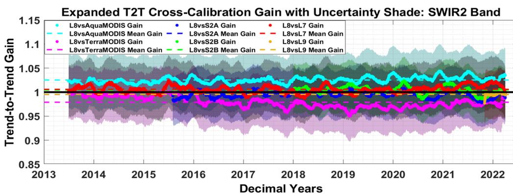
Figure 25. Expanded T2T cross-calibration gain of six sensor pairs for the SWIR2 band using EPICS Global. The shaded region shows uncertainty associated with each pair of sensors.
